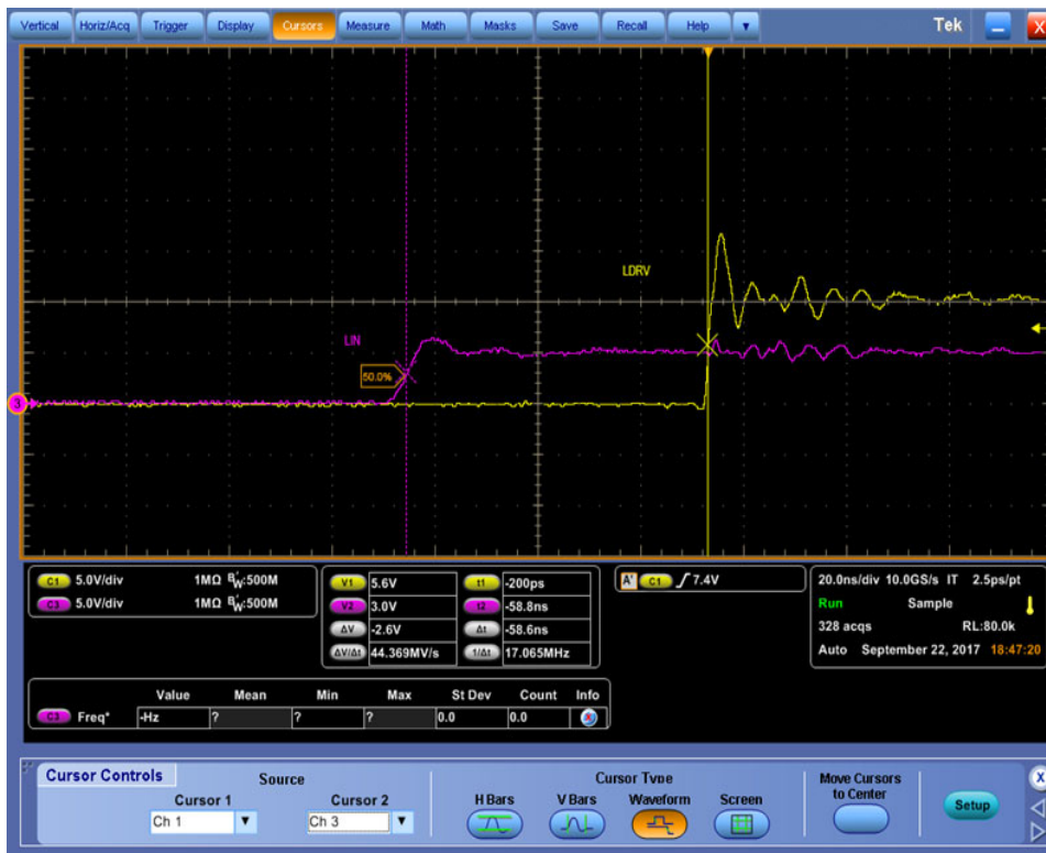
Figure 29. Low Side Turn-ON Propagation Delay (NCP51530A)
