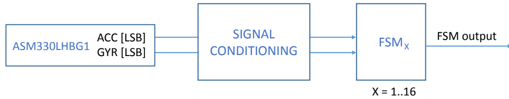
Figure 2. State machine in the ASM330LHBG1
