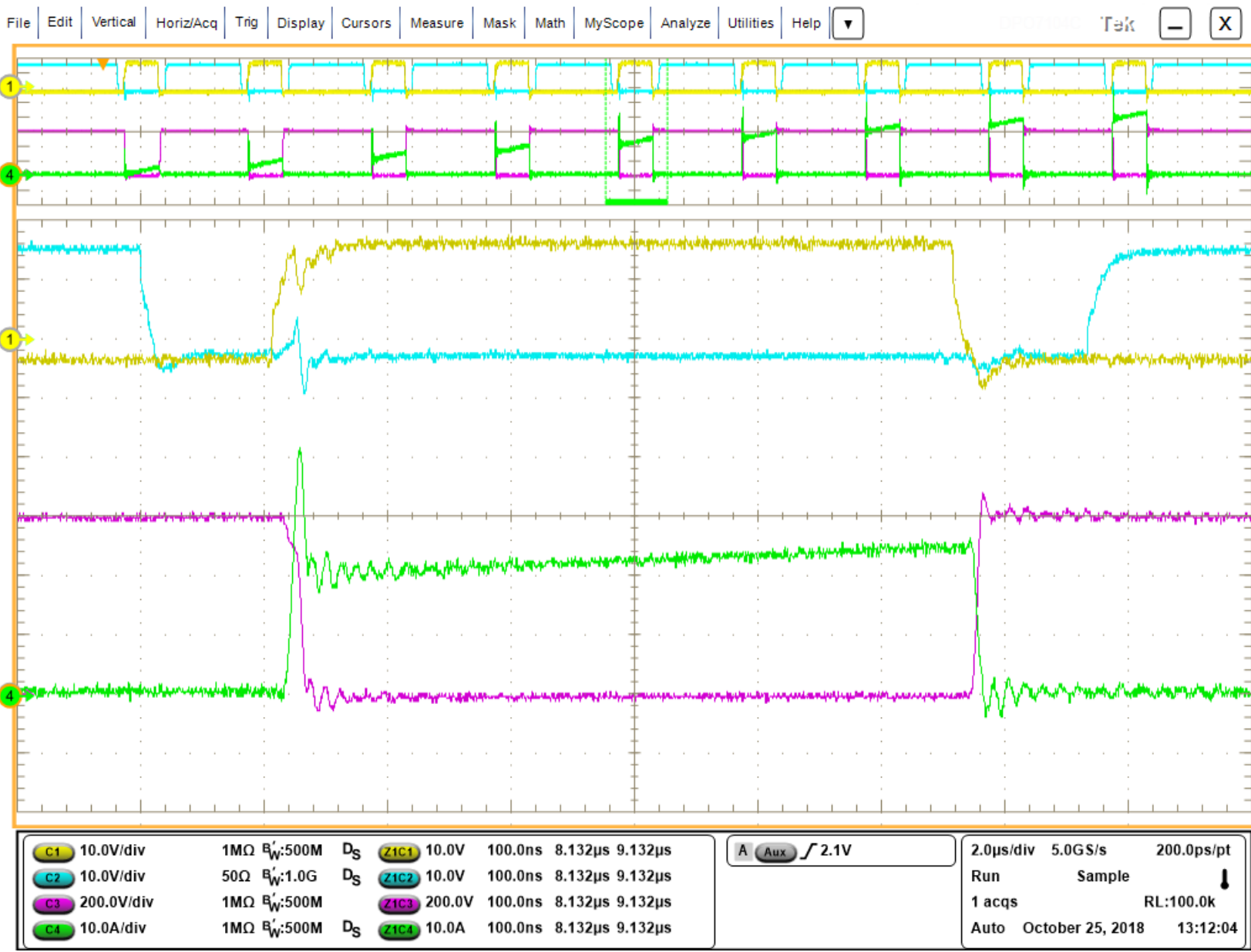
Figure 9-6. SiC MOSFET Switching Waveforms
