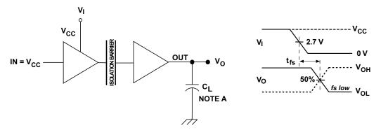
A.  $C_L = 15 \text{ pF}$  and includes instrumentation and fixture capacitance within ±20%.
