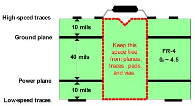
Figure 21. Recommended Layer Stack
