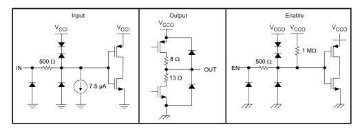
Figure 15. Device I/O Schematics
