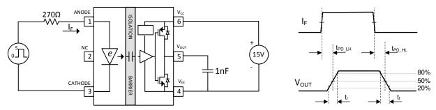
Figure 7-1. I<sub>F</sub> to V<sub>OUT</sub> Propagation Delay, Rise Time and Fall Time
