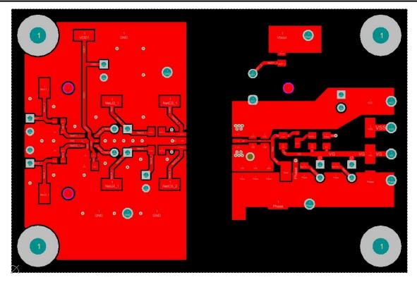
Figure 11-2. Top-Layer Traces and Copper
