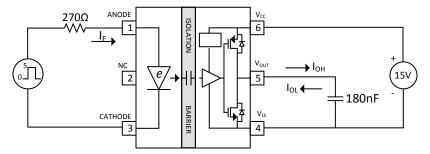
Figure 7-2. I<sub>OH</sub> and I<sub>OL</sub>
