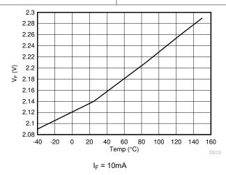
Figure 6-15. Forward voltage drop versus Temperature
