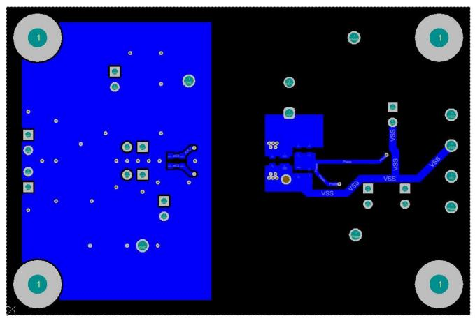
Figure 11-3. Bottom-Layer Traces and Copper (Flipped)
