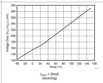
Figure 6-9. V<sub>OH</sub> (No Load) versus Temperature
