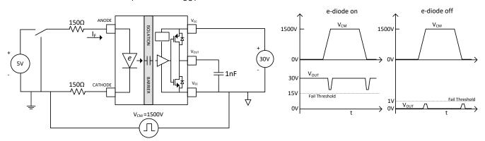
Figure 7-3. CMTI Test Circuit for UCC23313-Q1
