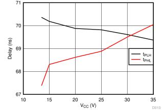
Figure 6-12. Propagation delay versus Supply voltage
