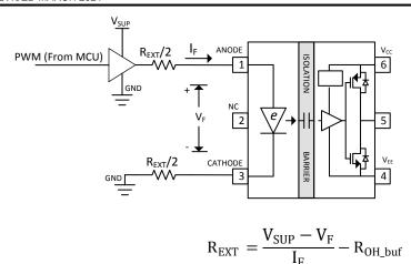
Figure 9-3. Configuration 2: Driving the input stage of UCC23313-Q1 with one Buffer and split resistors
