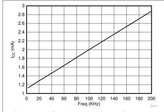
Figure 6-13. Supply current versus Frequency
