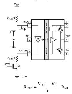
Figure 9-2. Configuration 1: Driving the input stage of UCC23313-Q1 with a single NMOS and split resistors
