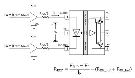
Figure 9-4. Configuration 3: Driving the input stage of UCC23313-Q1 with 2 buffers and split resistors
