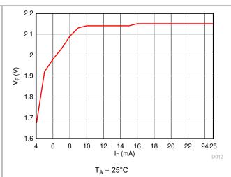
Figure 6-14. Forward current versus Forward voltage drop
