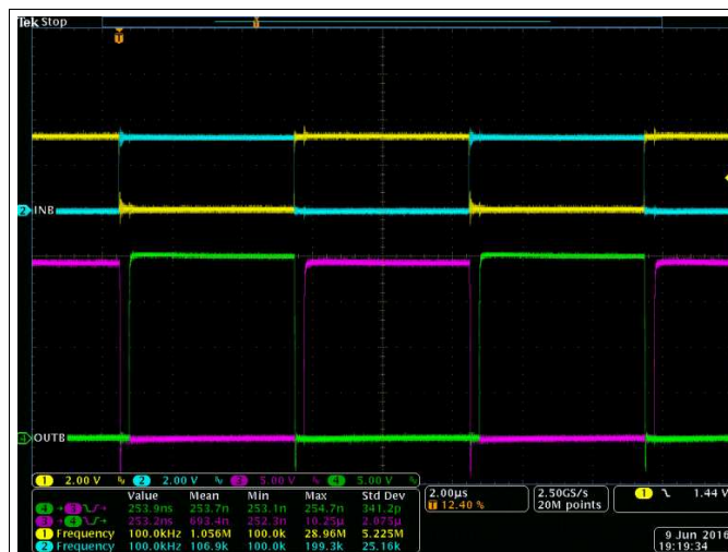
Figure 42. Bench Test Waveform for INA/B and OUTA/B
