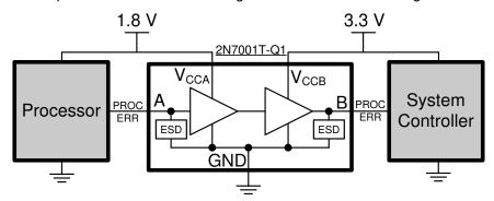
Figure 9-1. Processor Error Up Translation Application
