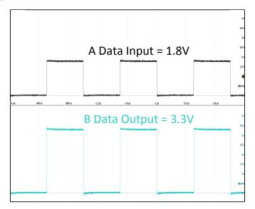
Figure 9-2. Up Translation (1.8 V to 3.3 V) at 1 MHz
