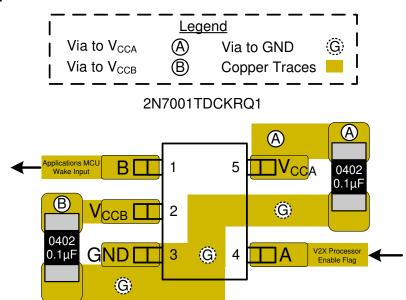
Figure 11-1. DCK Package Example Layout
