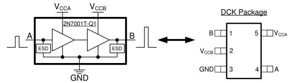
**Block Diagram and Pin Configuration**
