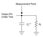
A. C<sub>L</sub> includes probe and jig capacitance.
