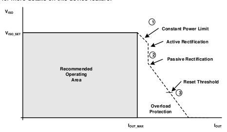
Figure 7-1. V<sub>ISO</sub> Load Recommended Operating Area Description
