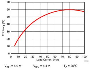
Figure 6-13. Power Supply Efficiency vs Load Current (I<sub>ISO</sub>)
