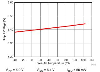
Figure 6-20. Isolated Supply Voltage (V<sub>ISO</sub>) vs Free-Air Temperature
