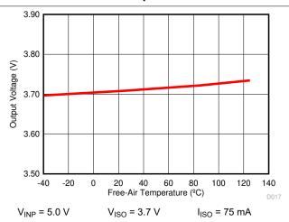
Figure 6-22. Isolated Supply Voltage (V<sub>ISO</sub>) vs Free-Air Temperature
