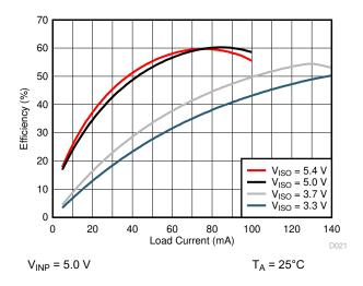
Typical Efficiency vs. Load
