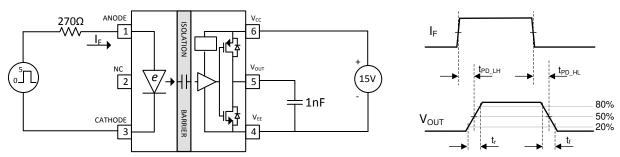
Figure 7-1. I<sub>F</sub> to V<sub>OUT</sub> Propagation Delay, Rise Time and Fall Time
