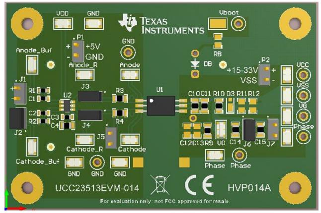
A. The location of the PCB cutout between primary side and secondary sides ensures isolation performance.
