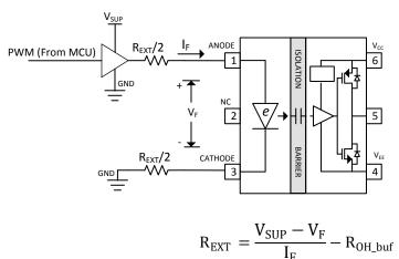
Figure 9-3. Configuration 2: Driving the input stage of UCC23313 with one Buffer and split resistors
