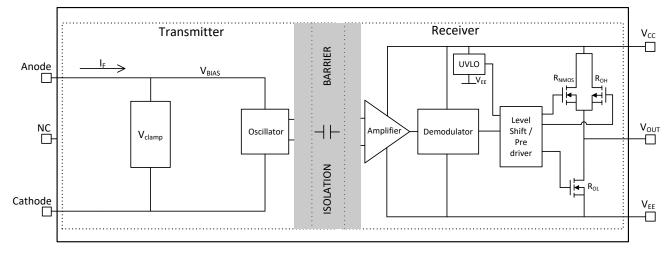
Figure 8-1. Conceptual Block Diagram of a Isolated Gate Driver with an Opto Emulated Input Stage (SO6 pkg)
