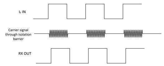
Figure 8-2. On-Off Keying (OOK) Based Modulation Scheme
