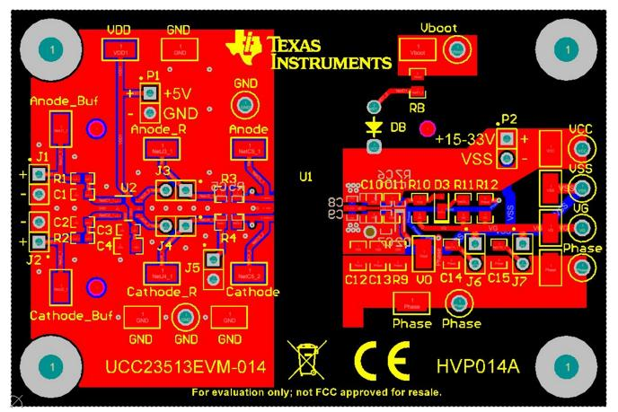
Figure 11-1 shows a PCB layout example with the signals and key components labeled.
