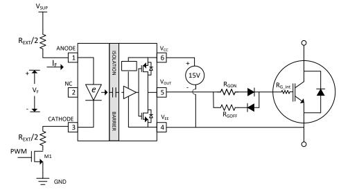
The circuit in Figure 9-1, shows a typical application for driving IGBTs.
