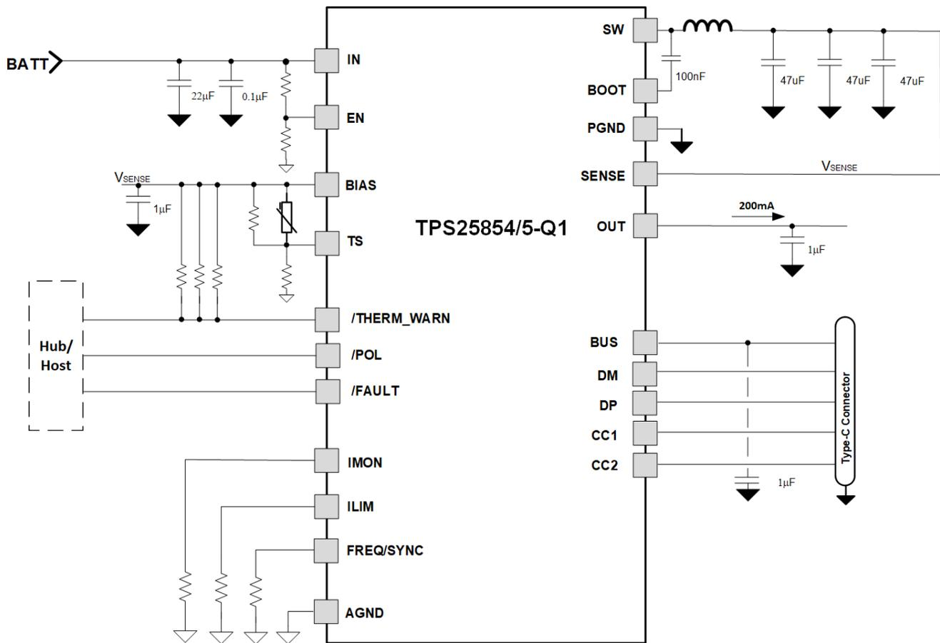
Figure 11-1. TPS2585x-Q1 Typical Application Circuit for 400-KHz  $f_{sw}$
