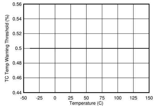
Figure 8-22. TS Temperature Wam Threshold vs Junction Temperature
