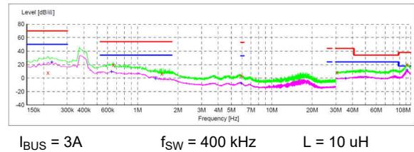
Figure 11-5. 400-KHz EMI Results (Without CM Filter)
