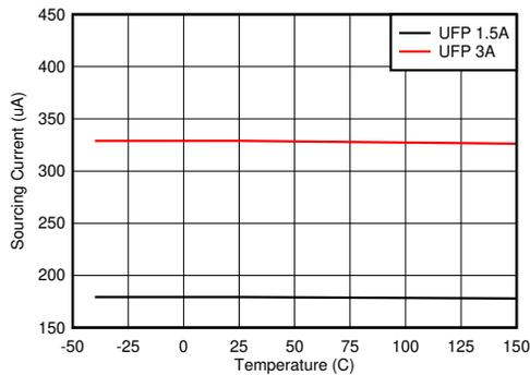
Figure 8-21. CC Sourcing Current vs Junction Temperature
