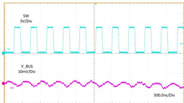
$I_{BUS} = 3 \text{ A}$   $f_{SW} = 2100 \text{ kHz}$
