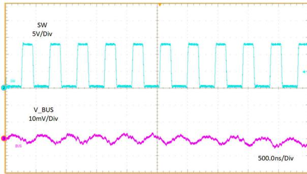
$I_{BUS} = 0.1 \text{ A}$        $f_{SW} = 2100 \text{ KHZ}$
