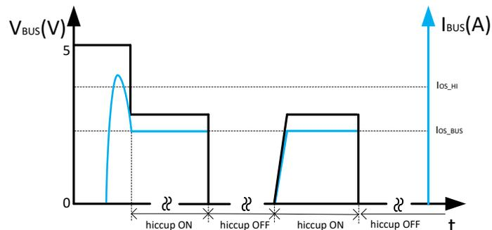
**Figure 10-7. BUS Overcurrent Protection: Two-Level Current Limit**
