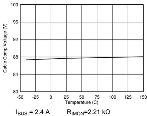
**Figure 8-15. Cable Compensation Voltage vs Junction Temperature**
