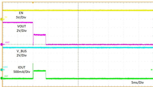
CC1 =  $R_d$     OUT = 5.1  $\Omega$     BUS NO LOAD
