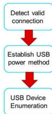
**Figure 10-13. Flow of DFP to UFP Configuration**
