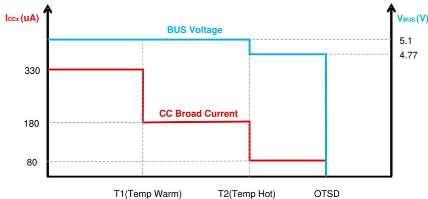
**Figure 10-11. TPS2585x-Q1 Behavior When Trigger Temp Warm/Hot Threshold**
