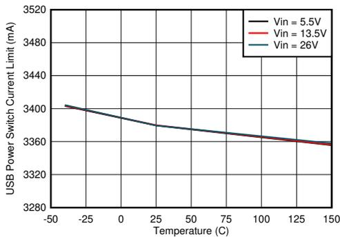
Figure 8-11. USB Power Switch Current Limit vs Junction Temperature
