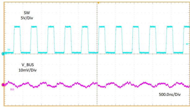
$I_{BUS} = 0 \text{ A}$        $f_{SW} = 2100 \text{ KHZ}$
