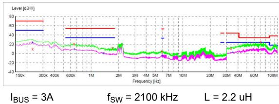
Figure 11-4. 2.1-MHz EMI Results (Without CM Filter)
