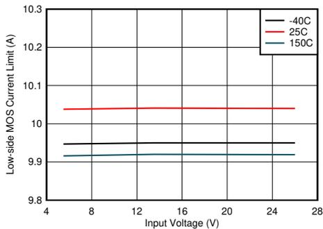
Figure 8-7. Low-side Current Limit vs Input Voltage
