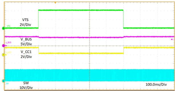
$V_{TS} = 0\text{ V to } 4\text{ V}$      $CC1 = R_d$      $CC2 = \text{OPEN}$
