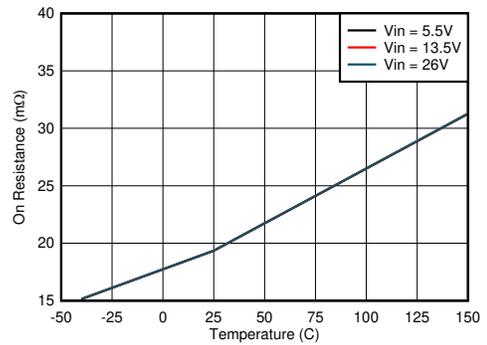
Figure 8-8. High-side MOSFET on Resistance vs Junction Temperature
