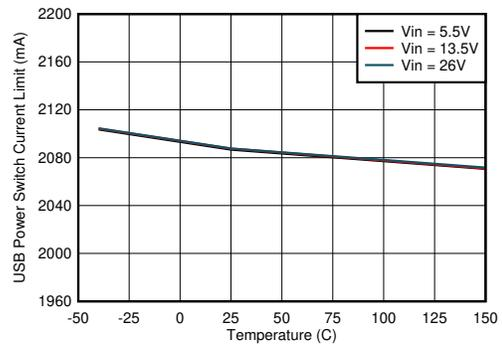
Figure 8-12. USB Power Switch Current Limit vs Junction Temperature
