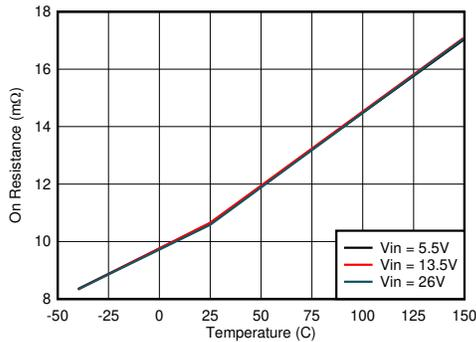
Figure 8-9. Low-side MOSFET on Resistance vs Junction Temperature
