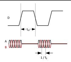
Figure 7-3. Measurement of Carrier Frequency
