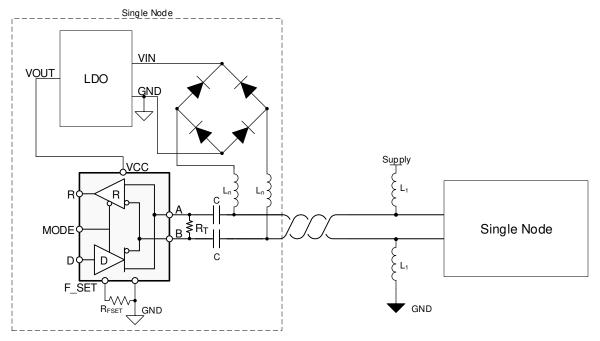
Figure 9-1. Typical power line network with 2 nodes
