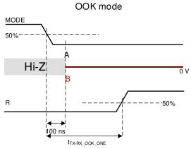
Figure 7-7. Transmit to Receive Mode Change with High Output
