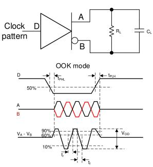
Figure 7-4. Measurement of Driver Switching Characteristics
