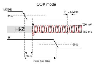
Figure 7-6. Transmit to Receive Mode Change with Low Output
