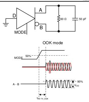
Figure 7-8. Receive to Transmit Mode Change
