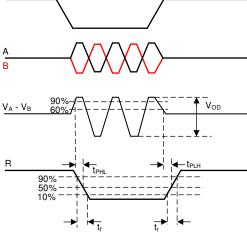
Figure 7-5. Measurement of Receiver Characteristics
