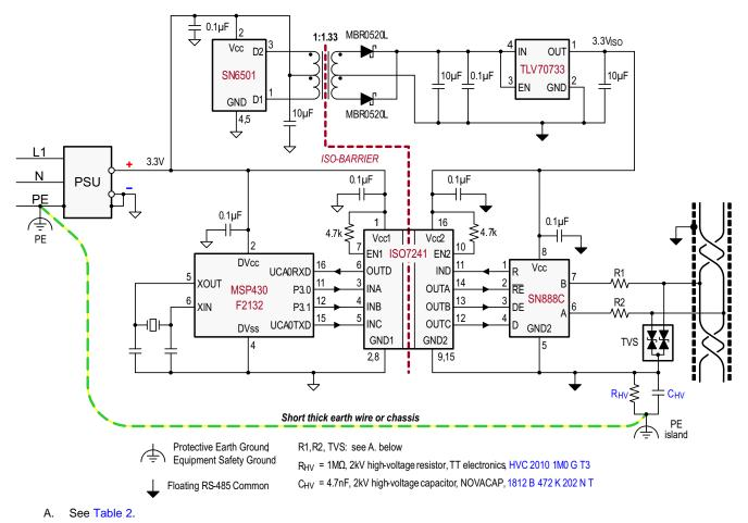
Figure 20. Isolated Bus Node With Transient Protection
