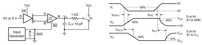
Figure 8. Measurement of Receiver Enable and Disable Times With Driver Enabled
