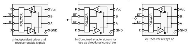
Figure 13. Transceiver Configurations
