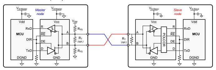
Figure 11. Point-To-Point Data Link With Cross-Wire Fault
