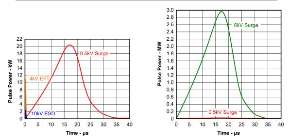
Figure 17. Power Comparison of ESD, EFT, and Surge Transients
