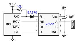
Figure 15. 3-V to 5-V Interface
