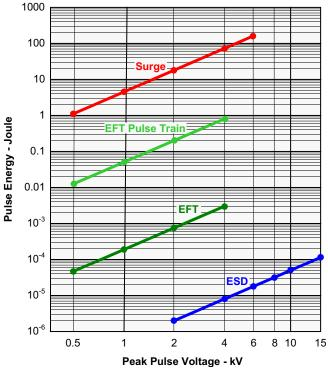
Figure 18. Comparison of Transient Energies
