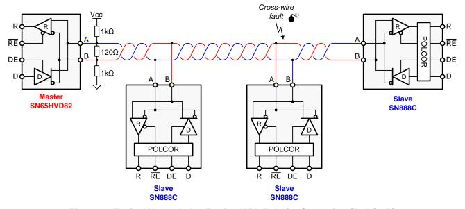
Figure 1. Typical Network Application With Polarity Correction (POLCOR)
