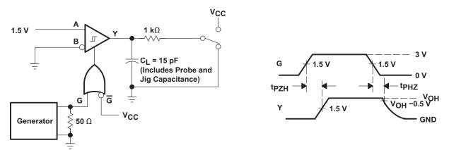
Generators: PRR = 1 MHz, 50% Duty Cycle, tr <6 ns, Z<sub>0</sub> = 50  $\Omega$
