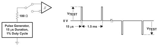
Figure 10. Test Circuit and Waveform, Transient Over-Voltage Test
