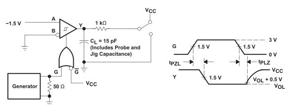
Generators: PRR = 1 MHz, 50% Duty Cycle, tr <6 ns, Zo = 50  $\Omega$
