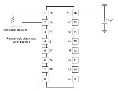
Figure 14. Layout with PCB Recommendations
