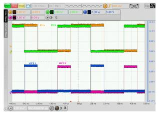
Figure 9-3. ISO6760L Interlock Diagram
