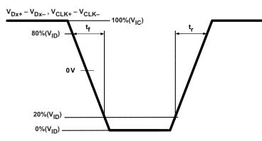
Figure 10. SubLVDS Differential Input Rise and Fall Time Defintion
