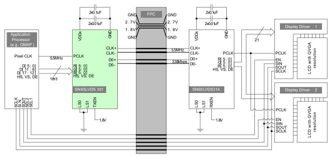
Figure 19. Example Dual-QVGA Display Application
