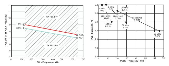
Figure 6. SN65LVDS314 PLL Bandwidth (also showing the SN65LVDS301 PLL bandwidth)
