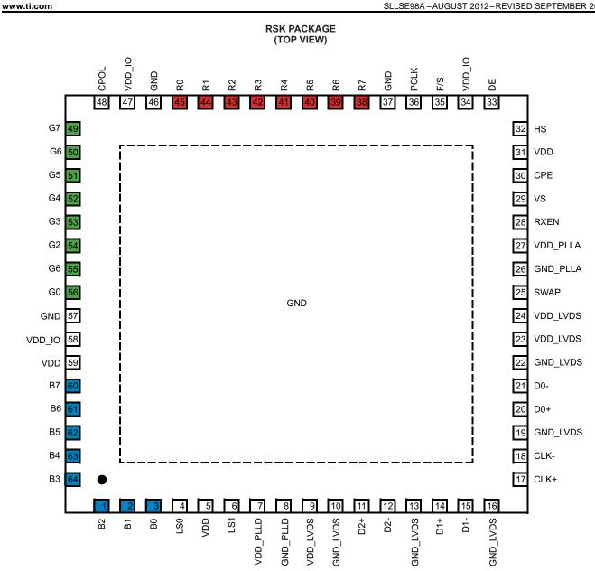
Figure 2. Pinout With SWAP PIN = VDD
