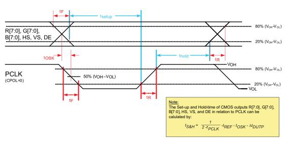
Figure 9. Output Rise/Fall, Setup/Hold Time
