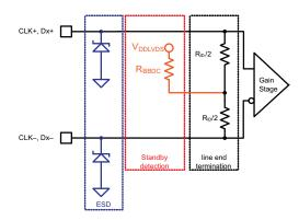
Figure 11. Equivalent Input Circuit Design
