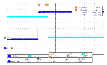
Figure 10-2. Measured Waveform Showing V<sub>IN0</sub> Pin and INT Pin Voltages
