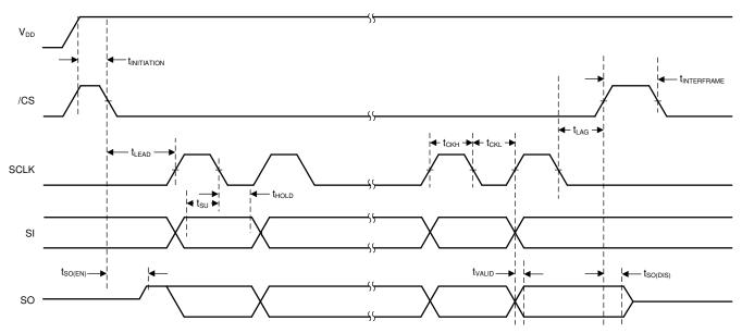
Figure 7-1. SPI Timing Parameters
