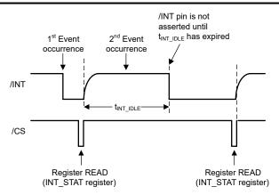
Figure 8-8.  $\overline{\text{INT}}$  Assertion Scheme With  $t_{\text{INT\_IDLE}}$
