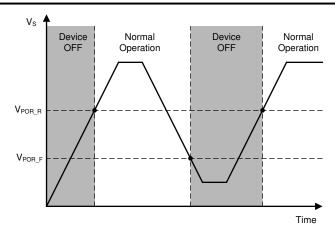
Figure 8-1. V<sub>S</sub> is Lowered Below The POR threshold, Then Ramped Back Up To Complete A POR Cycle
