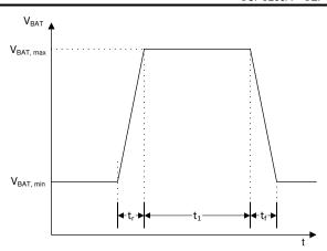
Figure 10-4. Voltage Profile to Test a Jump Start Event
