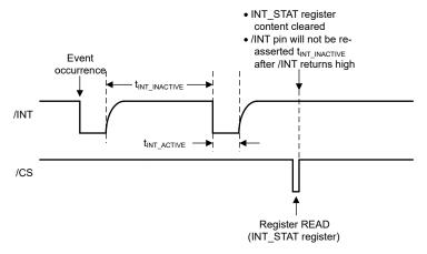
Figure 8-7. Dynamic INT Assertion Scheme With INT\_STAT Register Read During t<sub>INT INACTIVE</sub>
