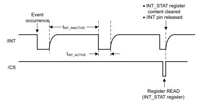
Figure 8-6. Dynamic INT Assertion Scheme With INT\_STAT Register Read During t<sub>INT ACTIVE</sub>
