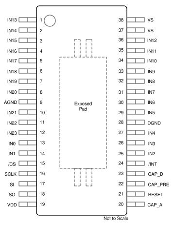
Figure 5-1. DCP (TSSOP) Package, 38-Pin, Top View
