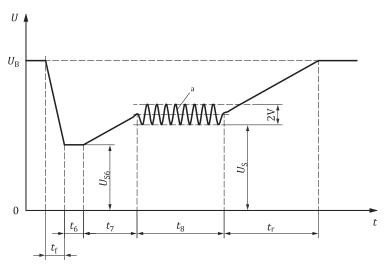
Figure 10-6. Voltage Profile to Test a Cranking Event
