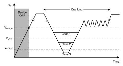
Figure 8-2. TIC10024-Q1 Operation At Various V<sub>S</sub> Voltage Levels
