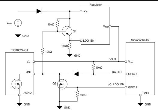
Figure 8-9. INT Connection to Support Microcontroller Wake-Up
