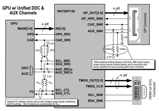
Figure 24. GPU with a Unified AUX/DDC Configuration
