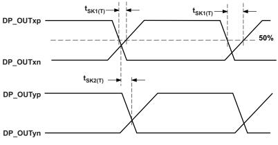
Figure 3. HDMI/DVI Sink TMDS Output Skew Measurements
