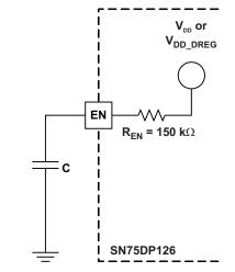
Figure 22. EN Input from Active Controller
