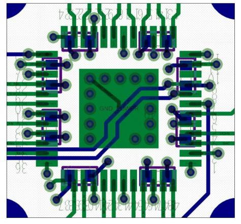
Figure 38. Thermal PAD Grounding
