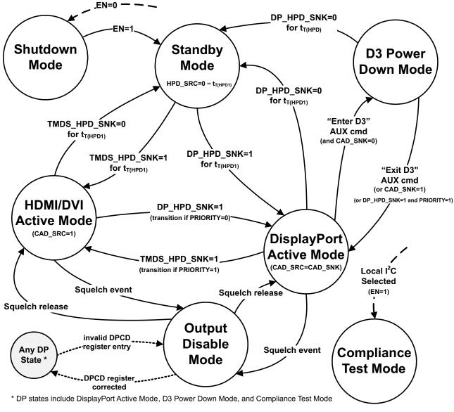
Figure 26. SN75DP126 Operating Modes Flow Diagram
