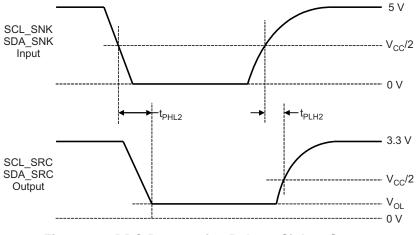
Figure 14. DDC Propagation Delay – Sink to Source
