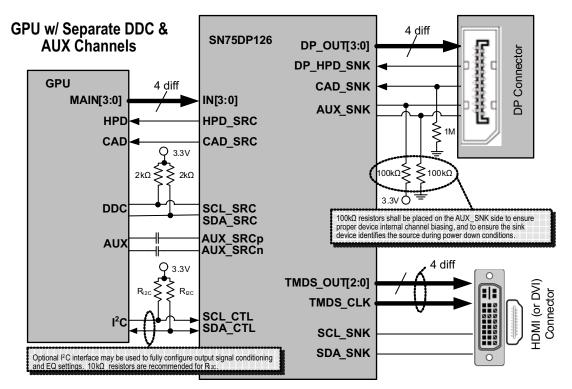
Figure 25. GPU with Separate DDC and AUX Channels
