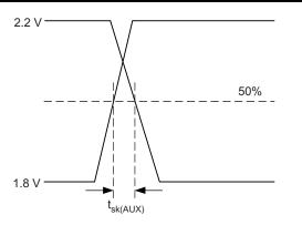
Figure 11. AUX Skew Measurement
