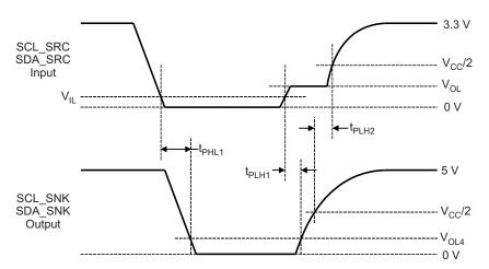
Figure 13. DDC Propagation Delay – Source to Sink
