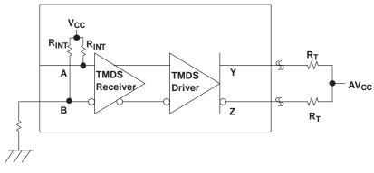
Figure 16. TMDS Input Fail-Safe Recommendation
