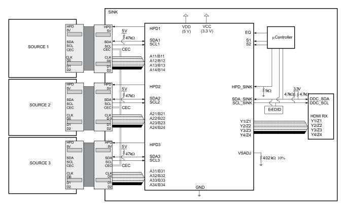
Figure 18. Three-Port HDMI Enabled DTV with TMDS351 – CEC Commands Passing Through
