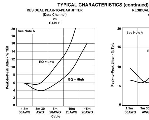
A. 1080p 10-Bit, V<sub>CC</sub> = AV<sub>CC</sub> = 3.3 V, T<sub>A</sub> = 25°C, R<sub>VSADJ</sub> = 4.02 kΩ, See Figure 6, Clock Channel = 185.6 MHz, Data Channel = 1.856 Gbps
