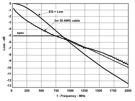
Figure 14. Frequency Response Compensation Curve at EQ = L
