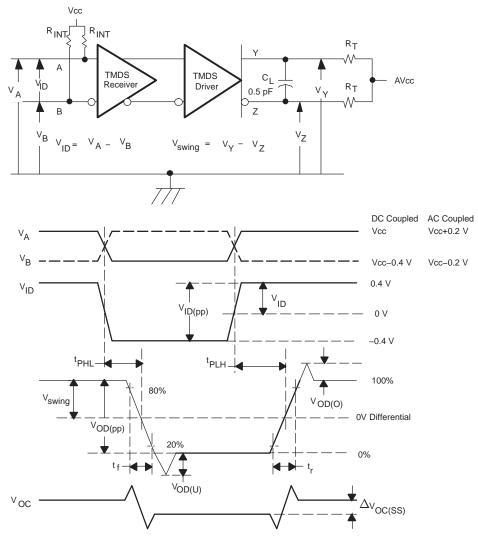
NOTE: All input pulses are supplied by a generator having the following characteristics: t<sub>r</sub> or t<sub>f</sub> < 100 ps, 100 MHz from Agilent 81250. C<sub>L</sub> includes instrumentation and fixture capacitance within 0.06 m of the D.U.T. Measurement equipment provides a bandwidth of 20 GHz minimum.
