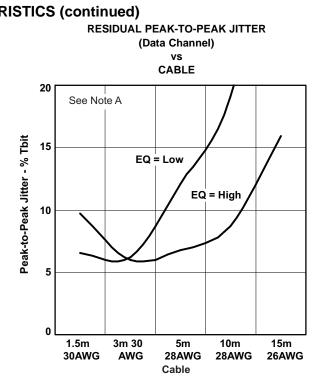
A. 1080p 12-Bit, V<sub>CC</sub> = AV<sub>CC</sub> = 3.3 V, T<sub>A</sub> = 25°C, R<sub>VSADJ</sub> = 4.02 kΩ, See Figure 6, Clock Channel = 222.8 MHz, Data Channel = 2.228 Gbps
