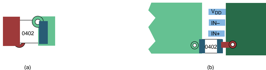
Figure 29. Typical Decoupling Capacitor Layouts
