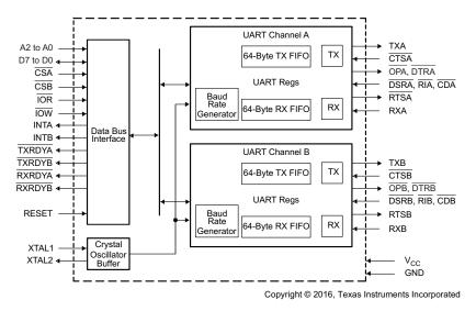
Figure 14. TL16C752D Functional Block Diagram
