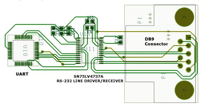
Figure 45. RS232 Channel Layout Example
