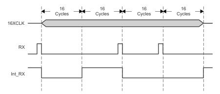
Figure 38. Positive RX Pulse Decode - Macro View
