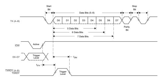
Figure 9. Transmit Timing in FIFO Mode
