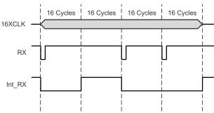
Figure 33. IrDA-SIR Decoding Scheme – Detailed Timing Diagram
