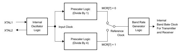
Figure 22. Prescaler and Baud Rate Generator Block Diagram
