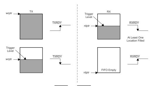
Figure 25. TXRDY and RXRDY in DMA Mode 1
