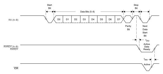
Figure 5. Receive Ready Timing in Non-FIFO Mode
