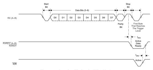
Figure 6. Receive Timing in FIFO Mode
