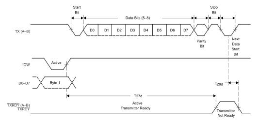
Figure 8. Transmit Ready Timing in Non-FIFO Mode
