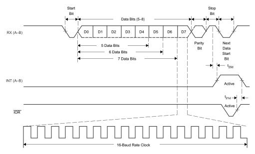
Figure 4. Receive Timing
