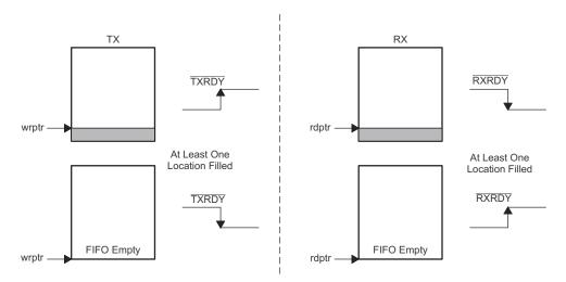
Figure 24. TXRDY and RXRDY in DMA Mode 0 or FIFO Disable
