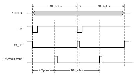
Figure 36. Recommended Strobing for Decoded Data
