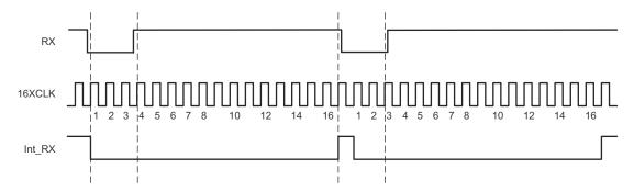
Figure 35. Timing Causing 1-Clock-Wide Pulse Between Consecutive Ones
