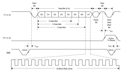
Figure 7. Transmit Timing
