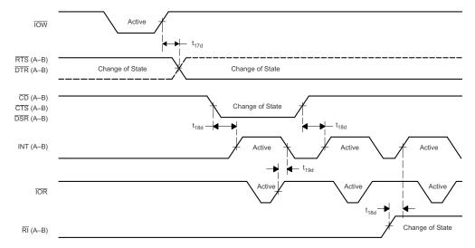
Figure 3. Modem or Output Timing
