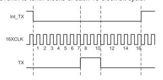
Figure 31. IrDA-SIR Encoding Scheme – Detailed Timing Diagram
