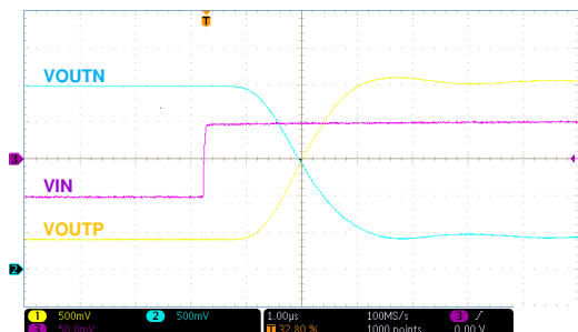
Figure 8-4. Step Response of the AMC1202
