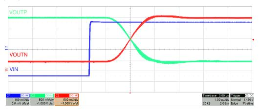
Figure 8-4. Step Response of the AMC1300B-Q1
