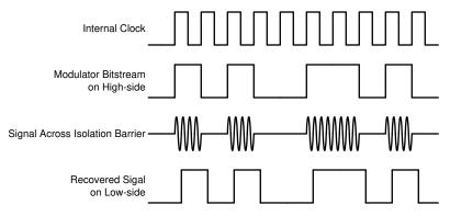
Figure 7-1. OOK-Based Modulation Scheme
