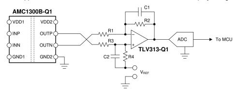
Figure 8-3. Connecting the AMC1300B-Q1 Output to a Single-Ended Input ADC
