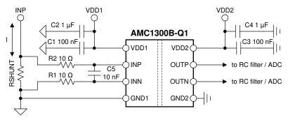
Figure 9-1. Decoupling of the AMC1300B-Q1
