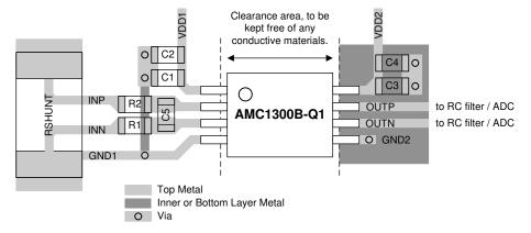
Figure 10-1. Recommended Layout of the AMC1300B-Q1
