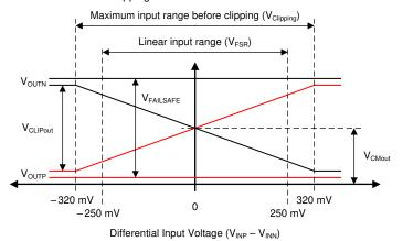
Figure 7-2. Output Behavior of the AMC1300B-Q1
