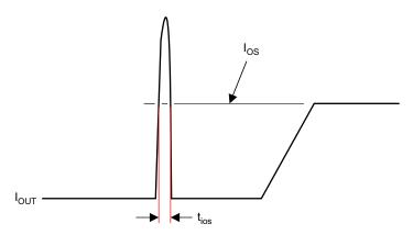
Figure 1. Output Short-Circuit Timing Diagram
