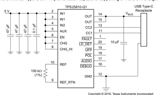
Figure 20. Type-C DFP Port Implementation Without BC 1.2 Support
