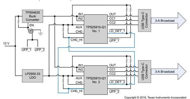
Figure 17. PPM and Power Wake Implemented
