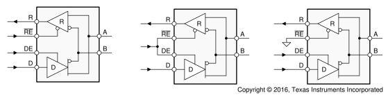
Figure 9-1. Half-Duplex Transceiver Configurations
