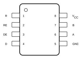
Figure 5-1. D (SOIC) Package, 8-Pin, Top View
