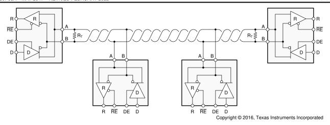
Figure 9-2. Typical RS-485 Network With Half-Duplex Transceivers
