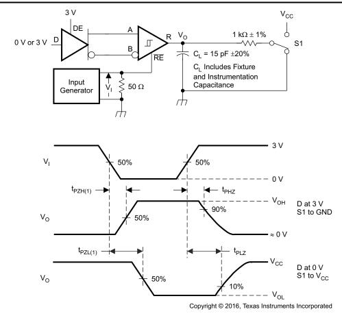
Figure 7-7. Measurement of Receiver Enable and Disable Times With Driver Enabled
