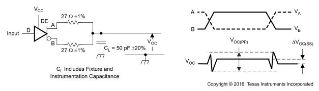
Figure 7-2. Measurement of Driver Differential and Common-Mode Output With RS-485 Load
