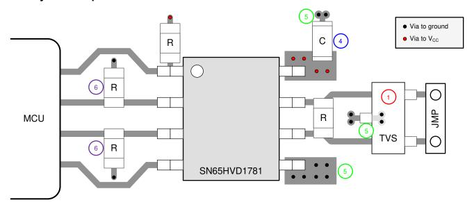
Figure 11-1. Half-Duplex Layout Example
