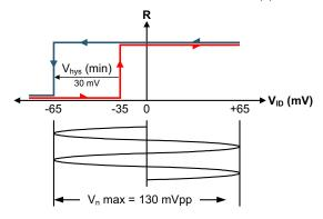
Figure 9-5. Noise Immunity Under Bus Fault Conditions
