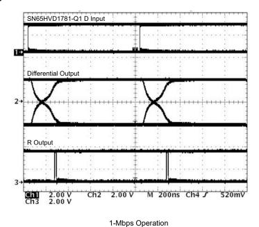
Figure 9-6. SN65HVD1781A-Q1 PRBS Data Pattern
