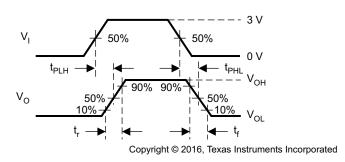
Figure 7-6. Measurement of Receiver Output Rise and Fall Times and Propagation Delays
