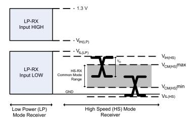
Figure 2. DSI Receiver Voltage Definitions
