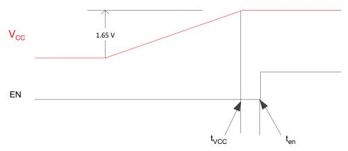
Figure 6. Cold-Start V<sub>CC</sub> Ramp Up to EN
