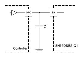
Figure 7. External Capacitor Controlled EN
