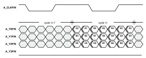
DE = Data Enable; A\_Y3P and A\_Y3N are output low; A\_Y3P and A\_Y3N are output low
