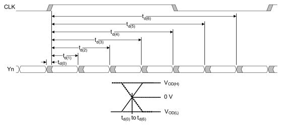
Figure 4. SN65DSI83-Q1 LVDS Timing Definitions
