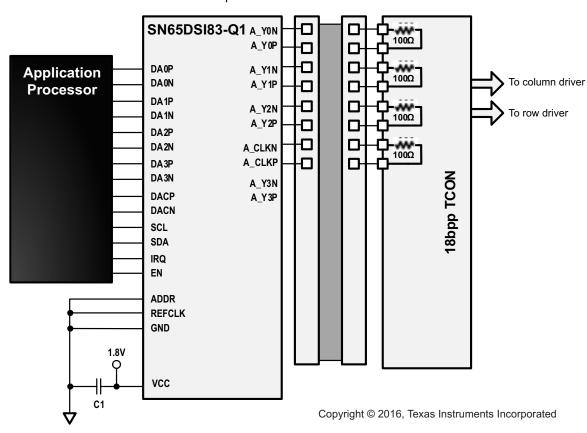
Figure 48. Typical WXGA 18-bpp Panel Application
