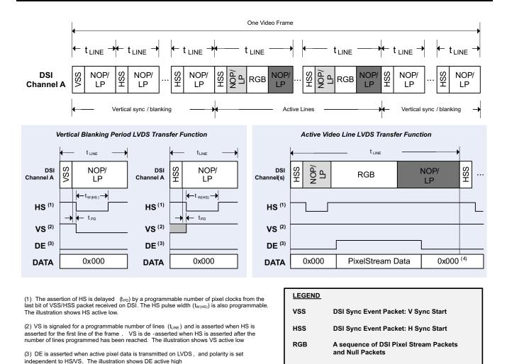
Figure 17. DSI Channel Transmission and Transfer Function
