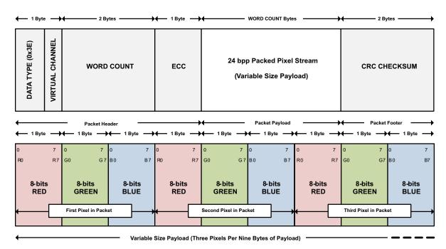
Figure 16. 24-bpp DSI Packet Structure
