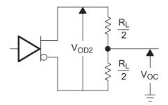
Figure 1. Driver Test Circuit,  $V_{\text{OD}}$  and  $V_{\text{OC}}$
