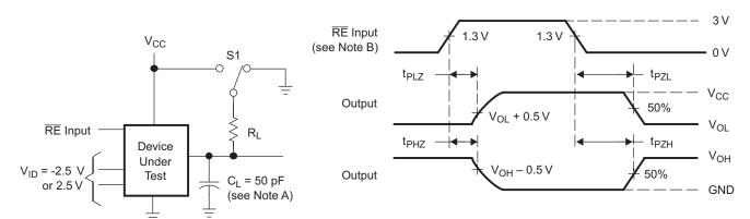
$t_{PZL},\,t_{PLZ}$  Measurement: S1 to V  $_{CC}$   $t_{PZH},\,t_{PHZ}$  Measurement: S1 to GND
