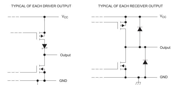
Figure 8. Schematic of Outputs
