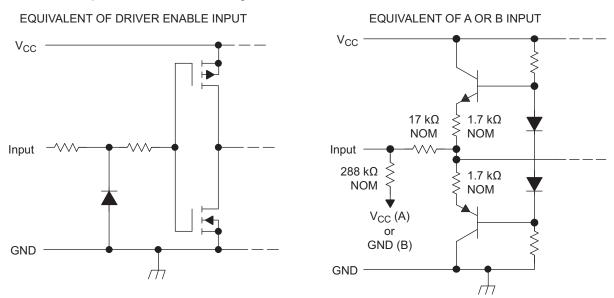
Figure 7. Schematic of Inputs
