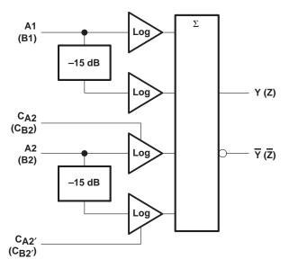
$\begin{array}{l} Y \propto \log A1 + \log A2; Z \propto \log B1 + \log B2 \\ \text{where: A1, A2, B1, and B2 are in dBV, 0 dBV = 1 V.} \\ C_{A2}, C_{A2'}, C_{B2}, \text{ and } C_{B2'} \text{ are detector compensation inputs.} \end{array}$
