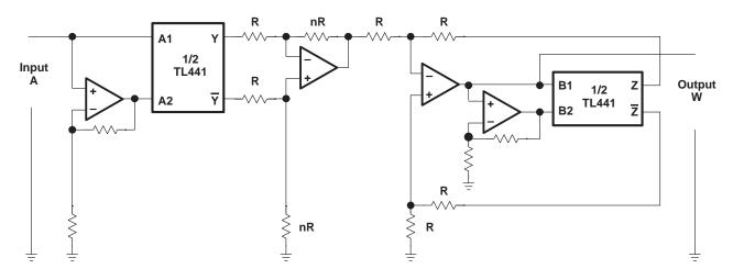
NOTE: R designates resistors of equal value, typically 2 k $\Omega$  to 10 k $\Omega$ . The power to which the input variable is raised is fixed by setting nR. Output W may need to be amplified to give the correct value.
