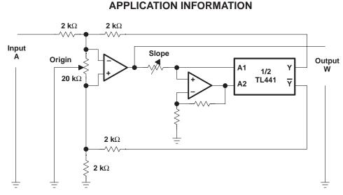
NOTE: Adjust the slope to correspond to the base "a". Exponential to any base: W = a.
