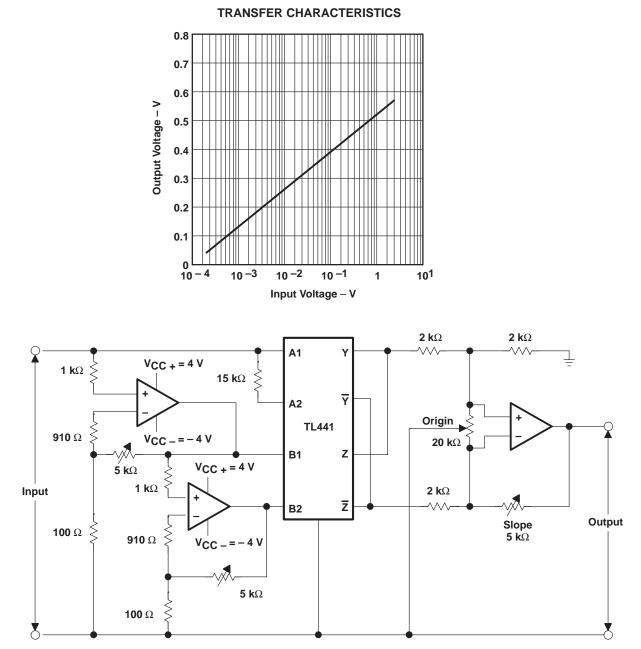
NOTES: A. Inputs are limited by reducing the supply voltages for the input amplifiers to  $\pm 4$  V. B. The gains of the input amplifiers are adjusted to achieve smooth transitions.
