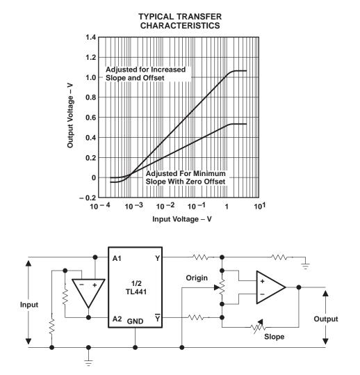
Figure 12. Output Slope and Origin Adjustment
