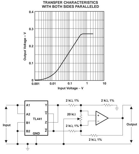
Figure 14. Utilization of Paralleled Inputs
