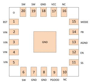
Figure 5-1. RJE Package 20-Pin VQFN (Top View)
