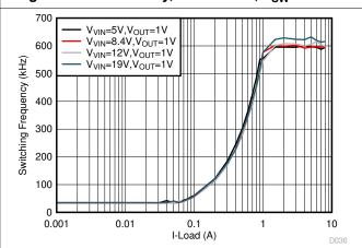
Figure 6-17. F<sub>SW</sub> Load Regulation, Eco-mode, F<sub>SW</sub> = 600 kHz
