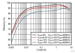
**Efficiency vs Output Current ECO-mode**
