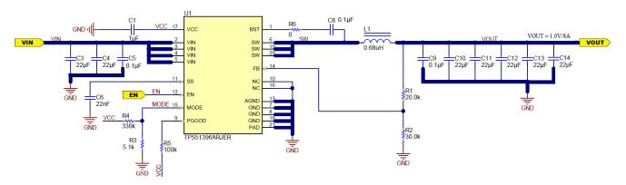
Figure 8-1. 1V/8A Reference Design with Eco-mode, Fsw = 600 kHz
