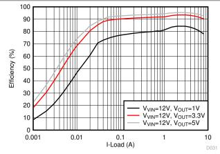
Figure 6-15. Efficiency, Eco-mode, F<sub>SW</sub> = 1 MHz
