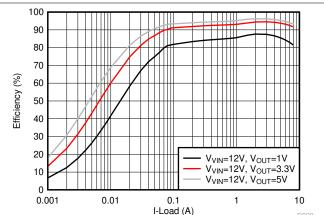
Figure 6-13. Efficiency, Eco-mode, F<sub>SW</sub> = 600 kHz
