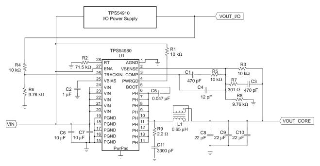
Analog and Power Grounds are Tied at the Power Pad Under the Package of IC
