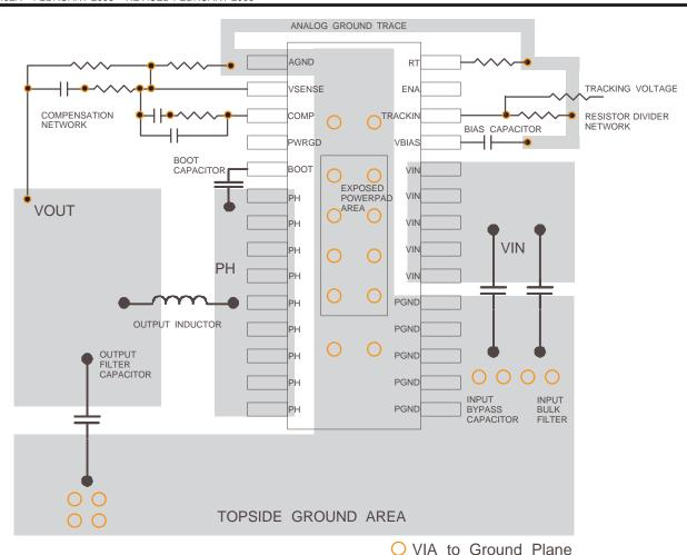
Figure 10. TPS54980 PCB Layout
