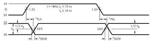
$t_{\text{PLH}}$  and  $t_{\text{PHL}}$  are measured to the respective 50% points.  $t_{\text{SKEW}}$  is the difference between propagation delays of the complementary outputs.
