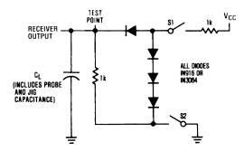
Figure 3. Receiver Propagation Delay Test Circuit
