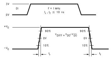
Figure 10. Driver Differential Transition Timing
