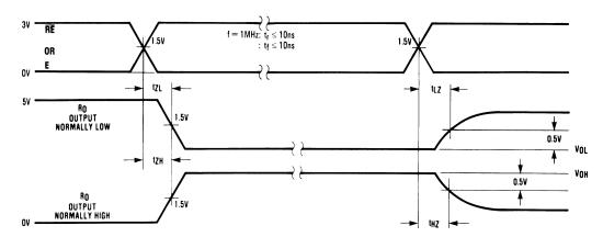
Figure 5. Receiver Enable/Disable Propagation Delay Timing
