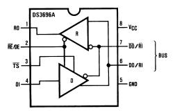
Figure 2. Top View (See Package Number D0008A)
