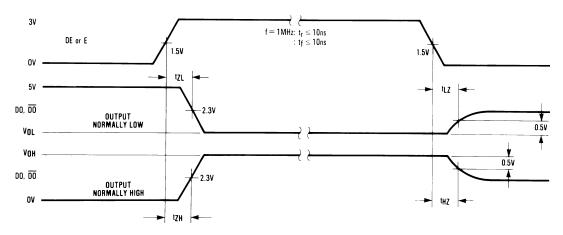
Figure 9. Driver Enable/Disable Propagation Delay Timing
