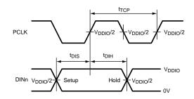
Figure 12. Serializer Setup/Hold Times
