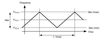
Figure 22. Spread Spectrum Clock Output Profile
