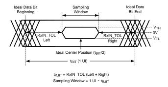
Figure 19. Receiver Input Jitter Tolerance
