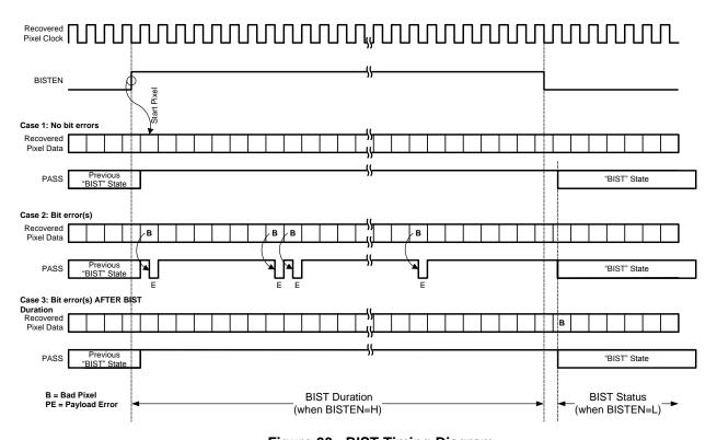
Figure 33. BIST Timing Diagram
