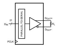
Figure 8. Serializer VOD DC Diagram
