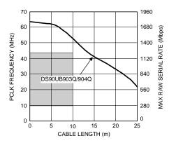
\*Note: Equalization is enabled for cable lengths greater than 7 meters
