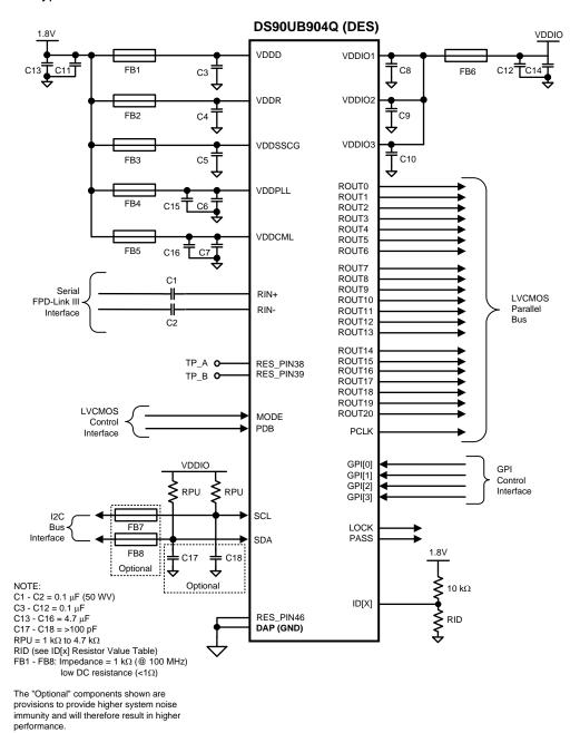
Figure 38. DS90UB904Q Typical Connection Diagram — Pin Control
