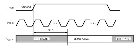
Figure 13. Serializer Data Lock Time
