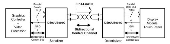
Figure 1. Typical Application Circuit
