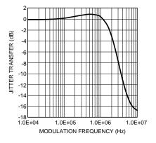
Figure 20. Typical Serializer Jitter Transfer Function Curve at 43 MHz
