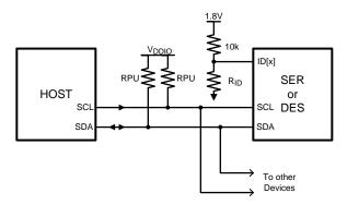
Figure 29. Bidirectional Control Bus Connection
