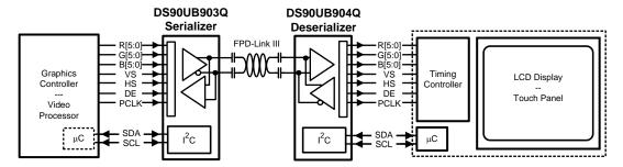
Figure 23. Typical Display System Diagram
