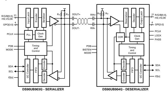
Figure 2. Block Diagram
