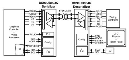
Figure 3. Application Block Diagram
