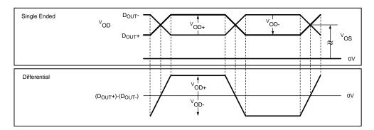
Figure 9. Serializer VOD DC Diagram
