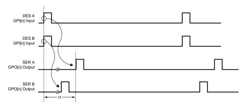
Figure 31. GPI/GPO Delta Latency
