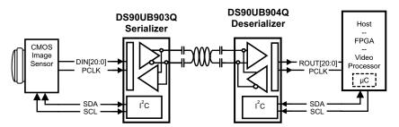
Figure 30. Typical Camera System Diagram
