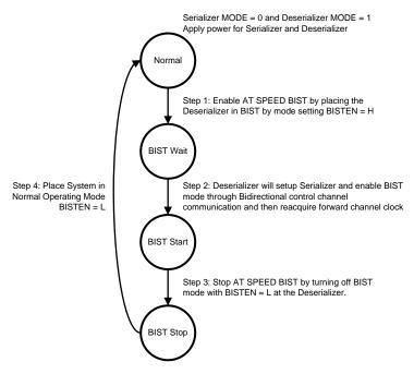
Figure 32. AT-SPEED BIST System Flow Diagram
