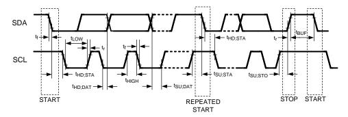
Figure 4. Bidirectional Control Bus Timing
