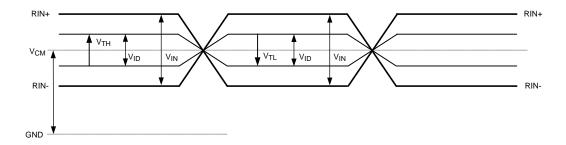
Figure 10. Differential VTH/VTL Definition Diagram
