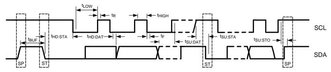
Figure 4. SMBus Timing Parameters
