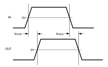
Figure 2. Propagation Delay Timing Diagram
