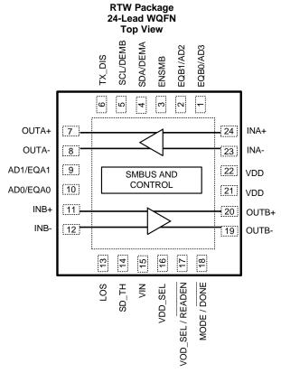
(1) The center DAP on the package bottom is the device GND connection. This pad must be connected to GND through multiple (minimum of 4) vias to ensure optimal electrical and thermal performance.
