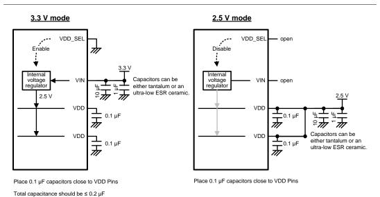
Figure 39. 3.3 V or 2.5 V Supply Connection Diagram
