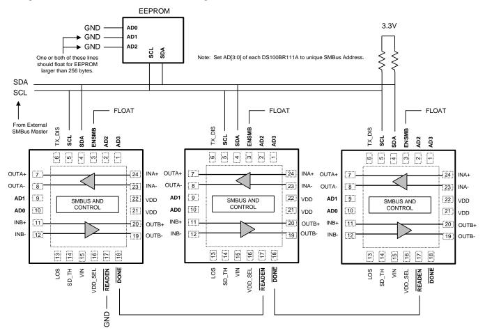
Figure 9. Typical Multi-Device EEPROM Connection Diagram
