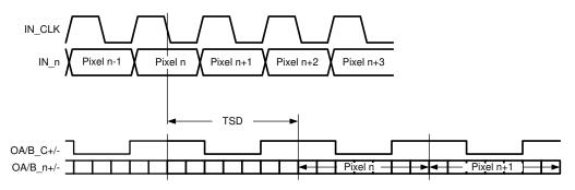
Figure 7-11. Single In, Single Out Mode Timing and Latency
