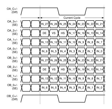
Figure 8-1. Dual Pixel / 24bpp LVDS Mapping
