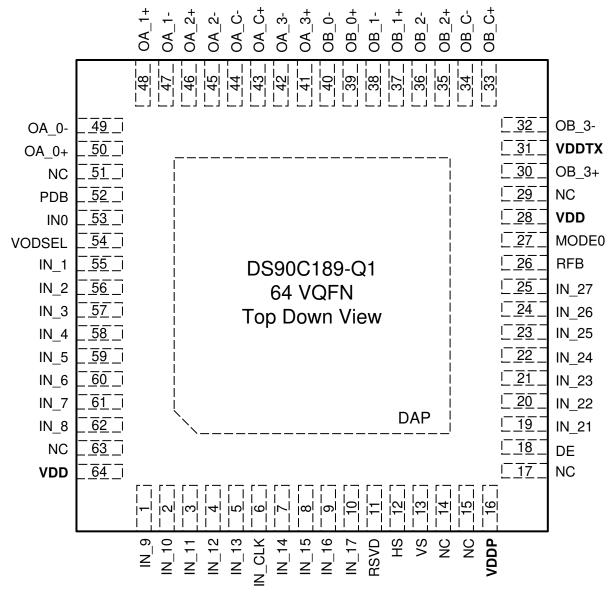
Figure 6-1. RTD Package 64-Pin VQFN Top View
