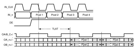
Figure 7-10. Single In, Dual Out Mode Timing and Latency
