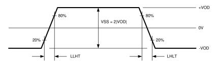
Figure 7-4. LVDS Output Transition Times
