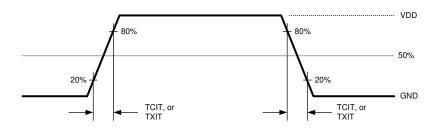
Figure 7-5. LVCMOS Input Transition Times
