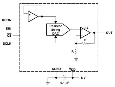
Figure 17. TLC5618 Typical Circuit
