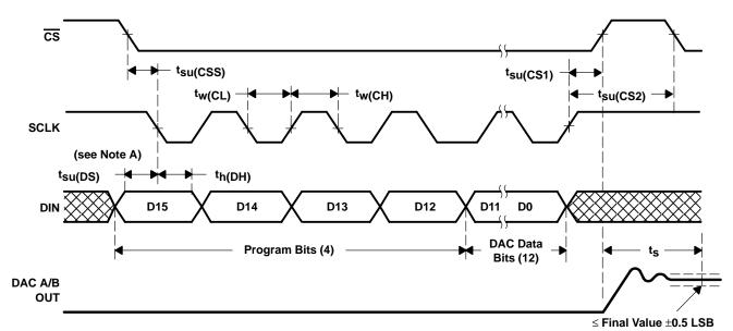
NOTE A: SCLK must go high after the 16th falling clock edge.
