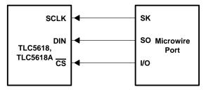
**Figure 23. Microwire Connection**
