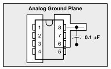
Figure 26. Power-Supply Bypassing
