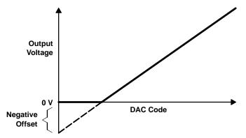
Figure 25. Effect of Negative Offset (Single Supply)
