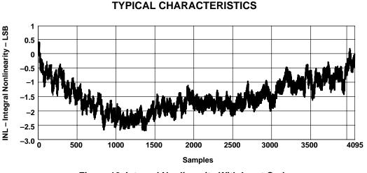
Figure 16. Integral Nonlinearity With Input Code
