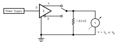
Figure 5. Differential Driver DC Open Test Circuit
