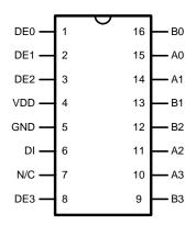
Figure 1. SOIC Package See Package Number D0016A
