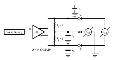
Figure 2. Differential Driver Test Circuit
