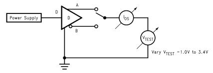
Figure 6. Differential Driver Short-Circuit Test Circuit
