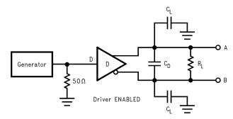
Figure 7. Driver Propagation Delay and Transition Time Test Circuit
