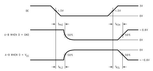
Figure 10. Driver TRI-STATE Delay Waveforms
