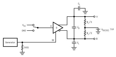
Figure 9. Driver TRI-STATE Delay Test Circuit
