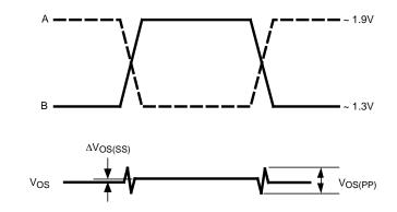
Figure 3. Differential Driver Waveforms
