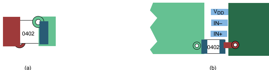
Figure 21. Typical Decoupling Capacitor Layouts
