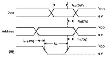
NOTES: A.  $t_r = t_f = 20$  ns over  $V_{DD}$  range.
