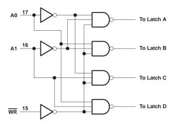
Figure 6. Input Control Logic
