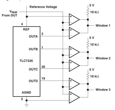
Figure 12. Overlapping Window Circuit
