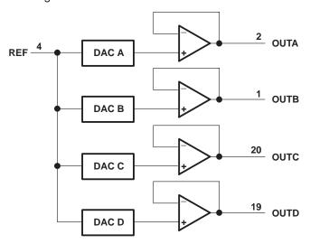
Figure 7. Unipolar Output Circuit
