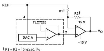
Figure 9. Bipolar Output Circuit
