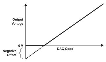
Figure 8. Effect of Negative Offset (Single Power Supply)
