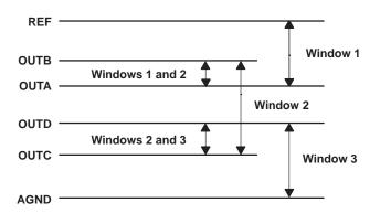
Figure 13. Overlapping Window Structure
