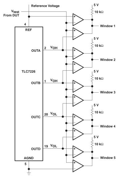
Figure 10. Logic Level Measurement
