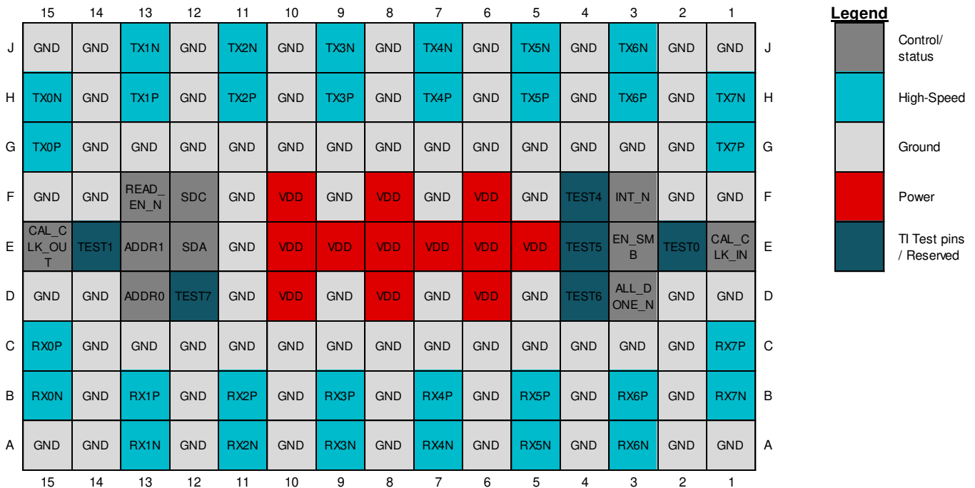
135-pin fcBGA, 0.8mm BGA pin pitch Top View
