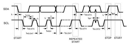
Figure 8. Serial Control Bus Timing Diagram
