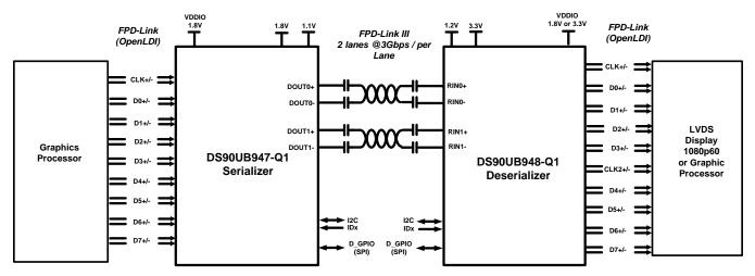
Figure 37. Typical System Diagram
