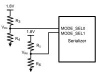
Figure 30. MODE\_SEL[1:0] Connection Diagram
