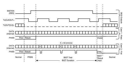
Figure 29. BIST Waveforms, in Conjunction With Deserializer Signals
