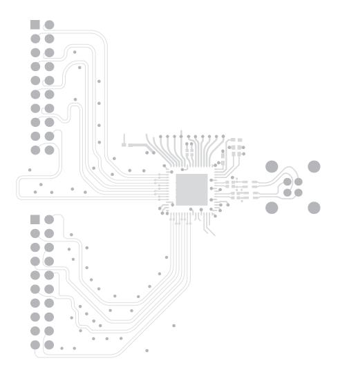
Figure 43. DS90UB947-Q1 Serializer Layout Example
