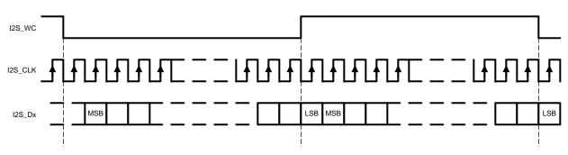
Figure 22. I2S Frame Timing Diagram
