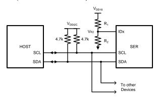
Figure 31. Serial Control Bus Connection
