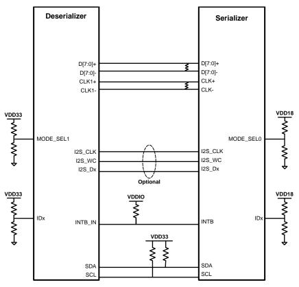
Figure 26. Repeater Connection Diagram
