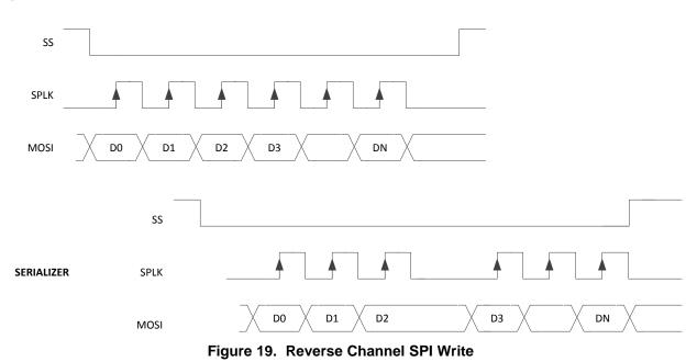
For Reverse Channel SPI reads, the SPI master must wait for a round-trip response before generating the sampling edge of the SPI clock. This is similar to operation in Forward channel mode. Note that at most one data/clock sample will be sent per back channel frame.
