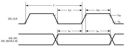
Figure 9. I2S Timing Diagram
