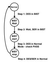
Figure 28. BIST Mode Flow Diagram
