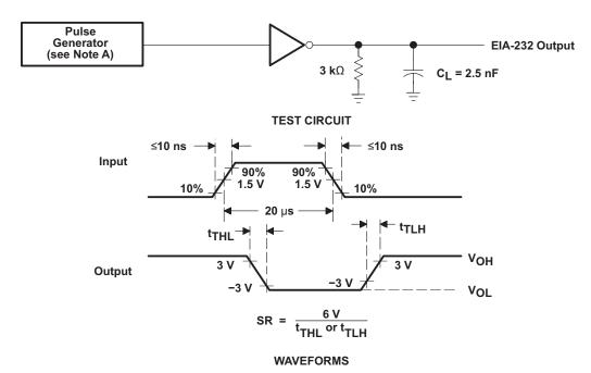
A. The pulse generator has the following characteristics:  $Z_0 = 50 \Omega$ , duty cycle  $\leq 50\%$ .
