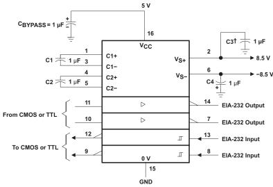
$\dagger$  C3 can be connected to V<sub>CC</sub> or GND.
