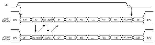
Figure 12. DATA0± and DATA1± Packet Format in According to CSI-2 Protocol for RGB888
