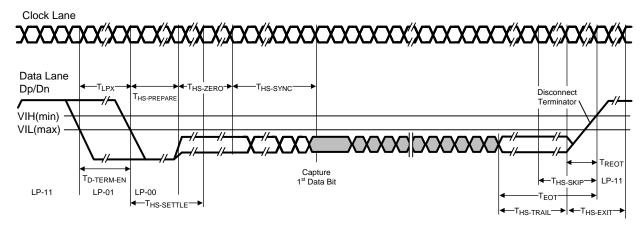
Figure 4. High-Speed Data Transmission Burst
