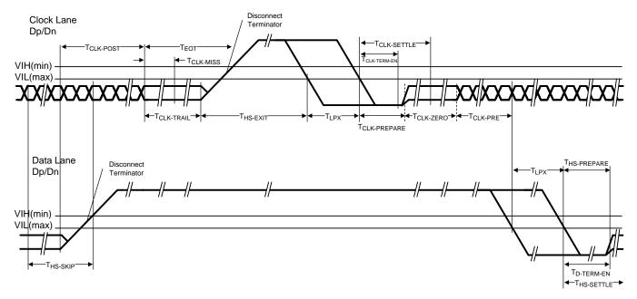
Figure 5. Switching the Clock Lane Between Clock Transmission and Low-Power Mode
