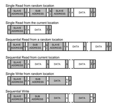
Figure 15. I2C or CCI Read or Write Operations
