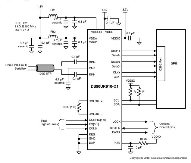
Figure 16. DS90UR910-Q1 Typical Connection Diagram — Pin Control
