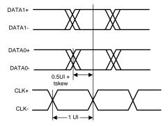
Figure 3. Clock and Data Timing in HS Transmission
