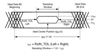
Figure 1. Receiver Input Jitter Tolerance
