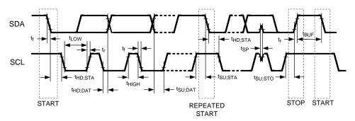
Figure 7. Serial Control Bus Timing Diagram
