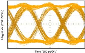
Figure 18. Loop-Through CML Output at 1.372-Gbps Serial Line Rate
