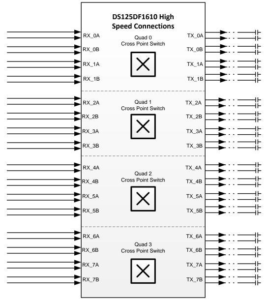
Figure 7. Typical Connection Diagram: High Speed Signals
