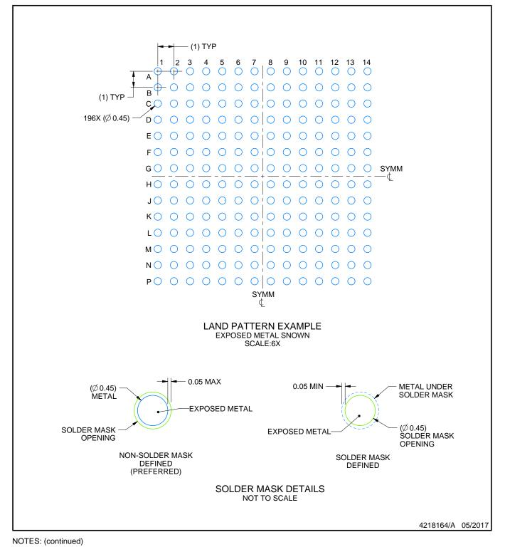
Final dimensions may vary due to manufacturing tolerance considerations and also routing constraints. For more information, see Texas Instruments literature number SPRU811 (www.ti.com/lit/spru811).
