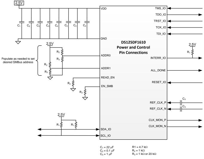
Figure 6. Typical Connection Diagram: Power and Control Pins
