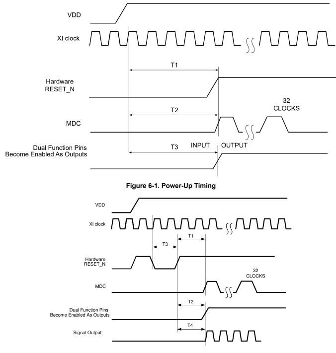
Figure 6-2. Reset Timing
