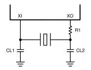
Figure 8-2. Crystal Oscillator Circuit
