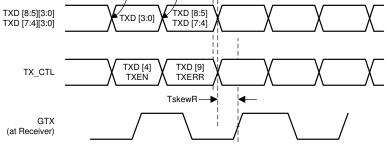
Figure 6-5. RGMII Transmit Multiplexing and Timing Diagram
