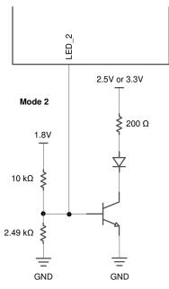
Figure 7-16. LED Operation From 1.8-V I/O VDD Supply
