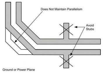
Figure 10-1. Avoiding Stubs in a Differential Signal Pair
