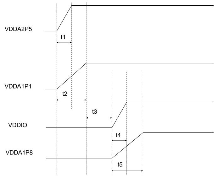
Figure 9-4. Three-Supply Sequence Diagram
