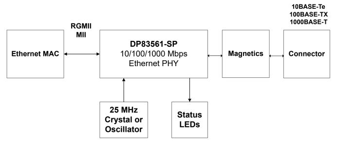
Figure 8-1. Typical Copper Ethernet Application
