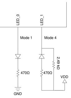
Figure 7-15. Example Strap Connections
