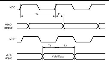
Figure 6-7. Serial Management Interface Timing
