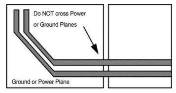
Figure 10-2. Differential Signal Pair-Plane Crossing
