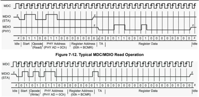
Figure 7-13. Typical MDC/MDIO Write Operation
