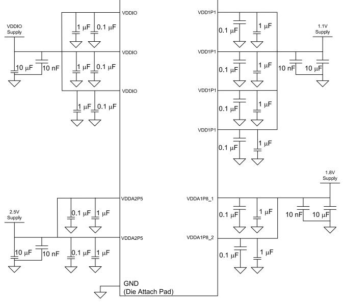
Figure 9-3 shows the connection diagram for the three-supply configuration.
