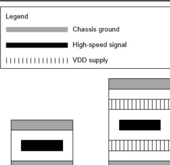
Figure 10-4. Alternative Layer Stack Up
