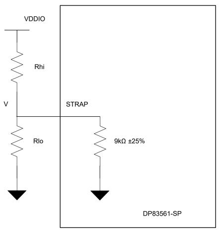
Figure 7-14. Strap Circuit
