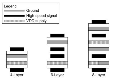
Figure 10-3. Recommended Layer Stack Up
