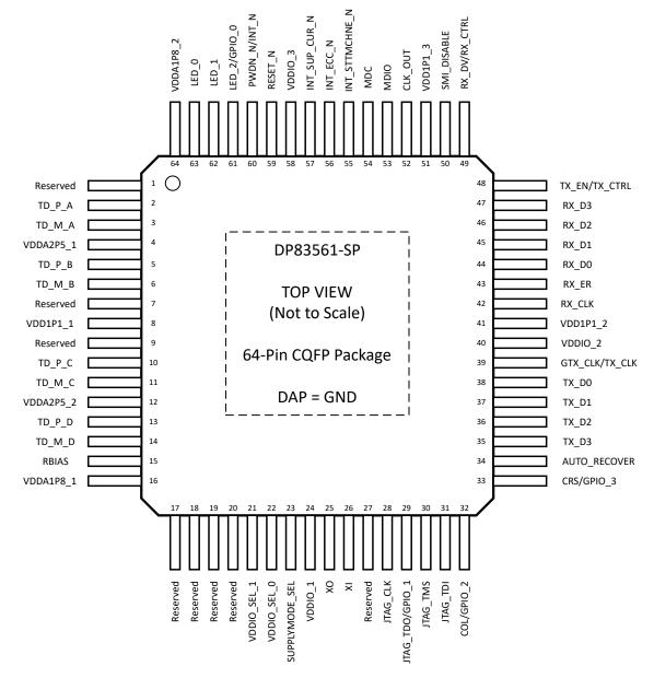
Figure 5-1. HBE Package 64-Pin CQFP Top View
