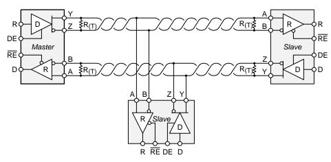
Figure 28. Typical RS-485 Network With Full-Duplex Transceivers
