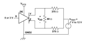
Figure 11. Driver V<sub>OD</sub> Test and Current Definitions
