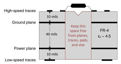
Figure 32. Recommended Layer Stack
