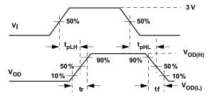
Figure 15. Driver Switching Test Circuit and Voltage Waveforms
