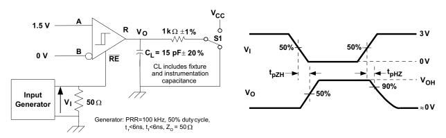
Figure 20. Receiver Enable Test Circuit and Waveforms, Data Output High
