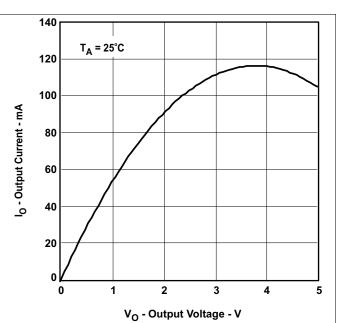
Figure 8. Receiver Low-Level Output Current vs Low-Level
