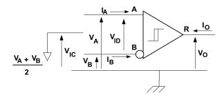
Figure 18. Receiver Voltage and Current Definitions
