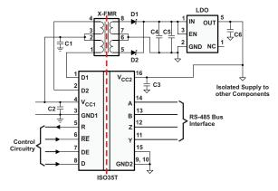
Figure 29. Typical Application Circuit
