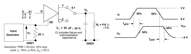
Figure 16. Driver High-Level Output Enable and Disable Time Test Circuit and Voltage Waveforms
