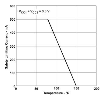
Figure 25. Thermal Derating Curve Per VDE
