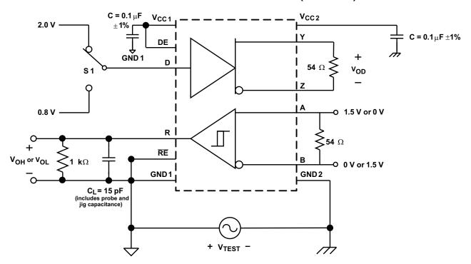
Figure 23. Common-Mode Transient Immunity Test Circuit
