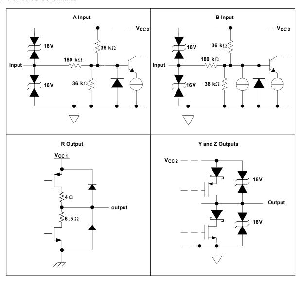
Figure 26. Equivalent Circuit Schematics
