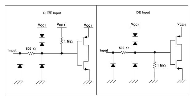
Figure 27. Equivalent Circuit Schematics
