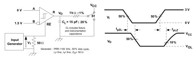
Figure 21. Receiver Enable Test Circuit and Waveforms, Data Output Low
