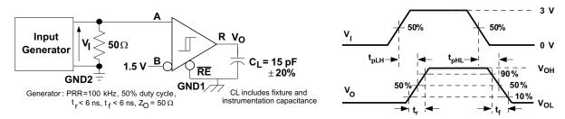
Figure 19. Receiver Switching Test Circuit and Waveforms
