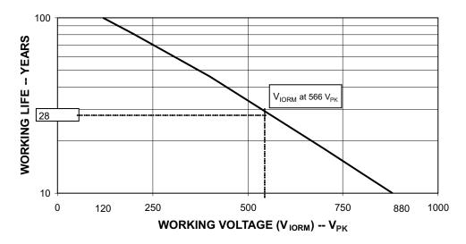
Figure 31. Time-Dependent Dielectric Breakdown Test Results
