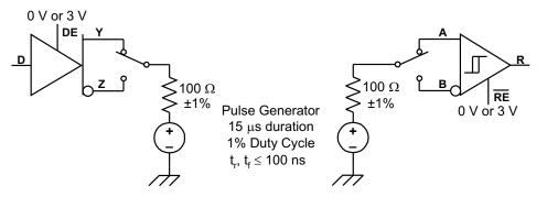
Figure 22. Transient Over-Voltage Test Circuit
