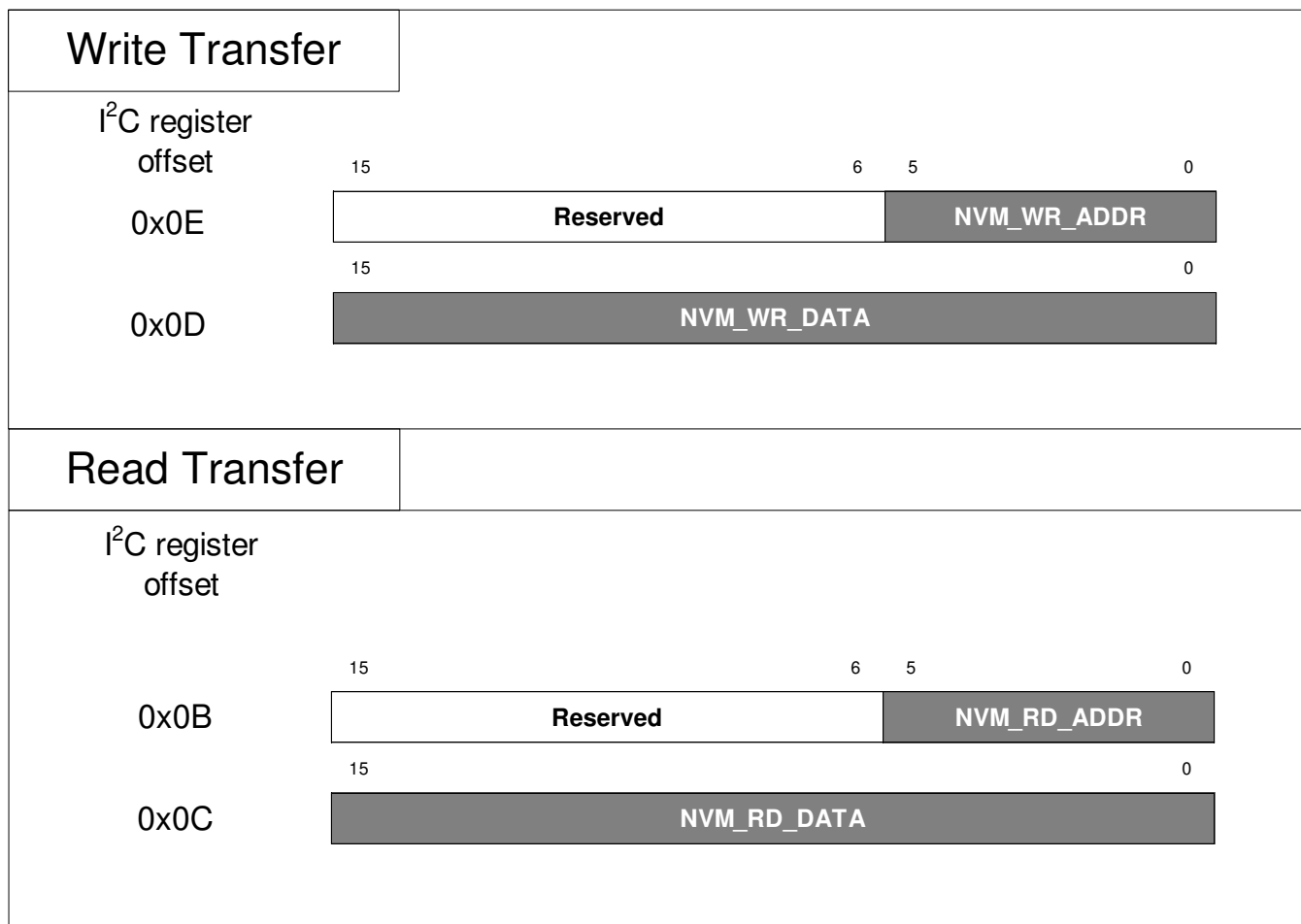
Figure 34. EEPROM Direct Access Using I 2 C
