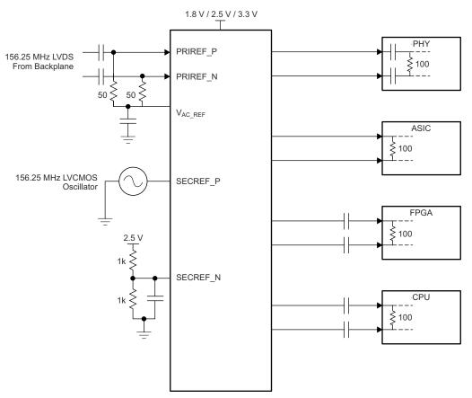
Figure 9-1. Fan-Out Buffer for Line Card Application
