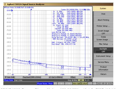
Figure 9-3. LMK1D1208 Output Phase Noise, 156.25 MHz, 46.4-fs RMS (12 kHz to 20 MHz)
