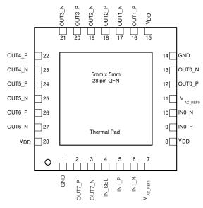
Figure 5-2. LMK1D1208: RHD Package 28-Pin VQFN Top View
