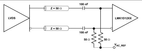
Figure 8-4. LVDS Clock Driver Connected to LMK1D120x Input (AC-Coupled)
