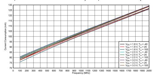
Figure 6-1. LMK1D1208 Current Consumption vs. Frequency
