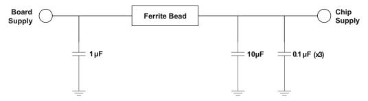
Figure 10-1. Power Supply Decoupling
