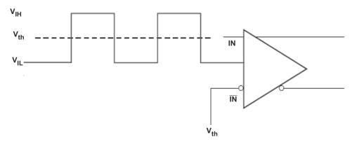
Figure 7-3. DC-Coupled LVCMOS Input During Device Test
