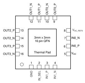
Figure 5-1. LMK1D1204: RGT Package 16-Pin VQFN Top View
