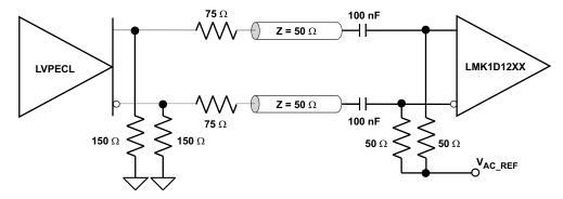
Figure 8-5. LVPECL Clock Driver Connected to LMK1D120x Input
