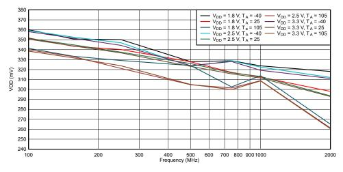
Figure 6-2. LMK1D1208 VOD vs. Frequency
