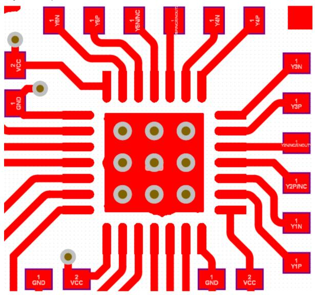
Figure 11-1. Recommended PCB Layout, Top Layer
