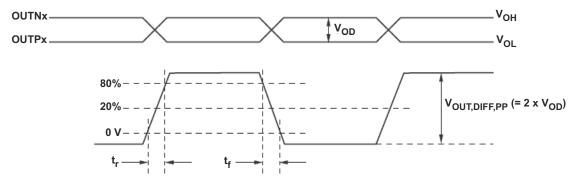
Figure 7-4. Output Voltage and Rise/Fall Time
