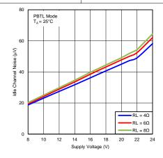
Figure 43. Idle Channel Noise vs Supply Voltage (PBTL Mode)
