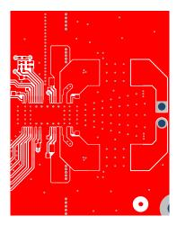
Figure 74. Layout Example (Mono) - Top Layer
