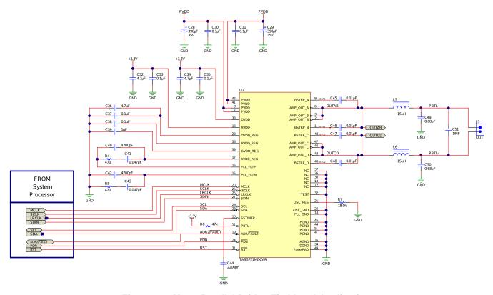
Figure 69. Mono Parallel Bridge Tied Load Application
