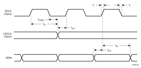
Figure 4. Serial Audio Port Timing
