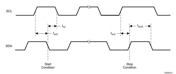
Figure 3. Start and Stop Conditions Timing
