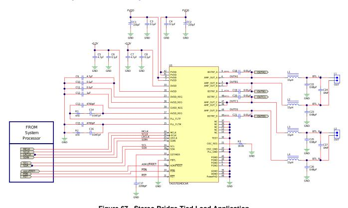
Figure 67. Stereo Bridge Tied Load Application
