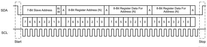
Figure 50. Typical I<sup>2</sup>C Sequence
