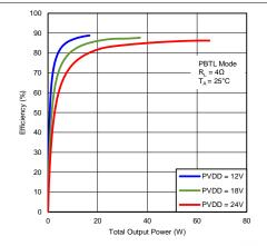
Total Output Power includes power delivered from both amplifier outputs. For instance, 40 W of total output power means 2 x 20 W, with 20 W delivered by one channel and 20 W delivered by the other channel.
