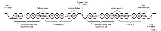
Figure 53. Single-Byte Read Transfer
