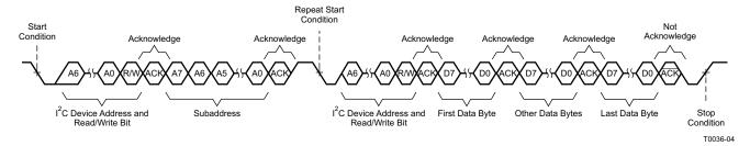
Figure 54. Multiple-Byte Read Transfer
