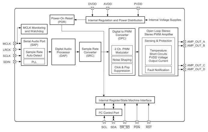
Figure 44. TAS5751M Functional Block Diagram
