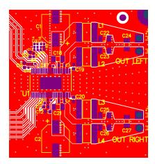
Figure 70. Layout Example (Stereo) - Top View Composite
