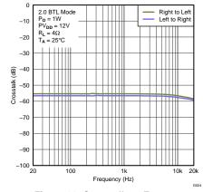
Figure 28. Crosstalk vs Frequency
