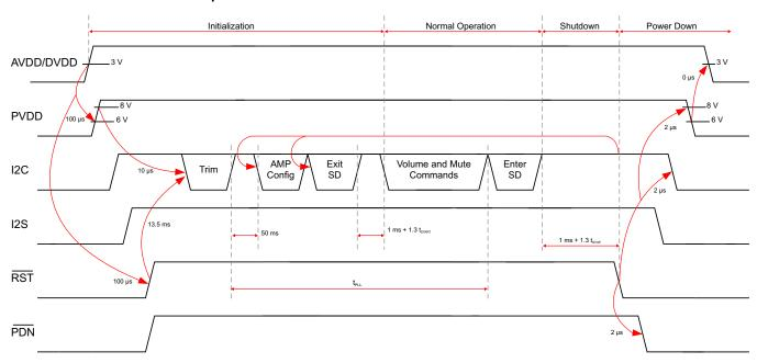
t<sub>PLL</sub> has to be greater than 240 ms + 1.3 t<sub>START</sub>, after the first trim command following AVDD/DVDD power-up. It does not apply to trim commands following subsequent resets. t<sub>START</sub>/t<sub>STOP</sub> = PWM start/stop time as defined in register 0x1A
