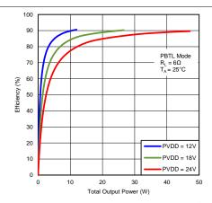
Total Output Power includes power delivered from both amplifier outputs. For instance, 40 W of total output power means  $2 \times 20$  W, with 20 W delivered by one channel and 20 W delivered by the other channel.
