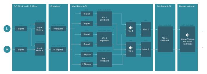
Figure 45. TAS5751M Audio Process Flow
