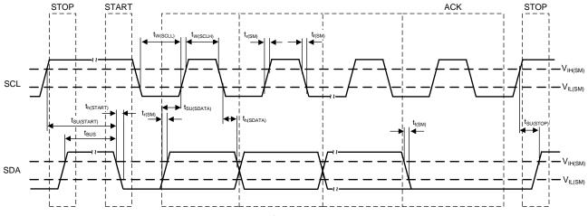
Figure 8. I<sup>2</sup>C Timing Diagram
