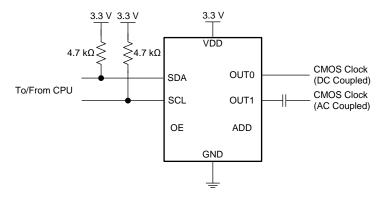
Figure 13. LMK61E0M Typical Application
