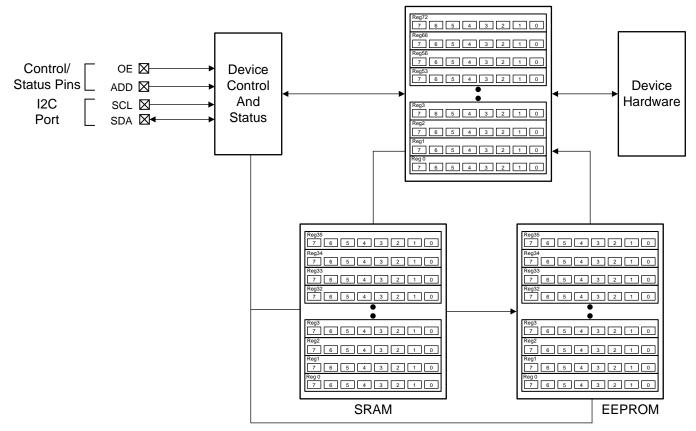
Figure 6. LMK61E0 Interface and Control Block
