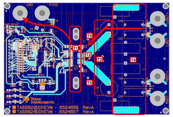
**Note T1**: Bottom and top layer ground plane areas are used to provide strong ground connections. The area under the IC must be treated as central ground, with IC grounds connected there and a strong via matrix connecting the area to bottom ground plane. The ground path from the IC to the power supply ground through top and bottom layers must be strong to provide very low impedance to high power and audio currents.
