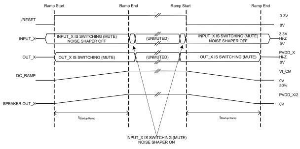
Figure 15. Start-Up and Shutdown Ramp
