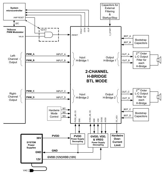
(1) Logic AND is inside or outside the microprocessor
