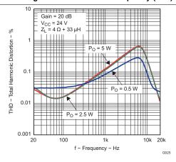
Figure 28. Total Harmonic Distortion vs Frequency (PBTL)
