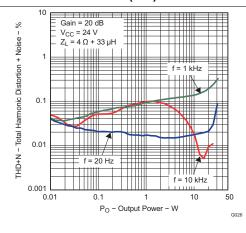
Figure 29. Total Harmonic Distortion + Noise vs Output Power (PBTL)
