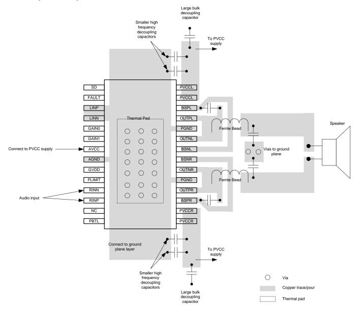
Figure 43. TPA3110D2-Q1 Layout Example for PBTL Output
