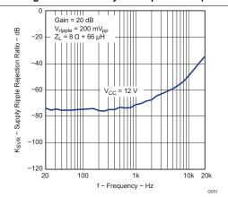
Figure 34. Supply Ripple Rejection Ratio vs Frequency (PBTL)
