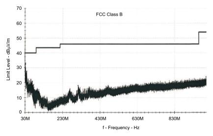
Figure 38. TPA3110D2-Q1 EMC Spectrum With FCC Class-B Limits
