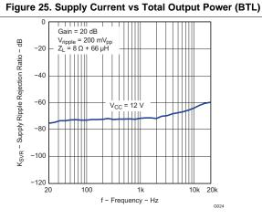
Figure 27. Supply Ripple Rejection Ratio vs Frequency (BTL)
