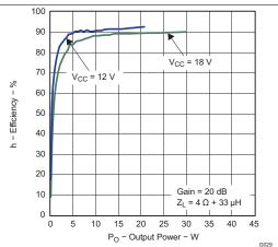
Figure 32. Efficiency vs Output Power (PBTL)
