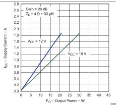
Figure 33. Supply Current vs Output Power (PBTL)
