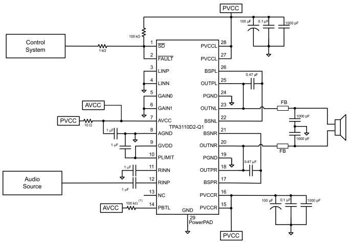
(1) A 100- $k\Omega$  resistor is needed if the PVCC slew rate is more than 10 V/ms.
