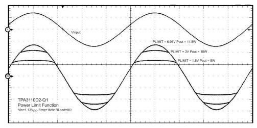
Figure 35. PLIMIT Circuit Operation
