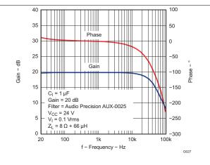
Figure 30. Gain/Phase vs Frequency (PBTL)
